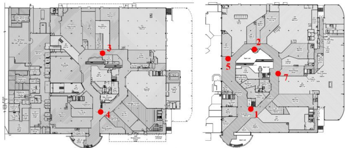
Figure 6: Sensors position in the common areas
