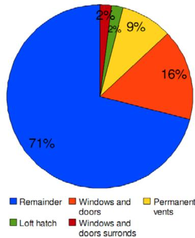
Figure 5. Air leakage paths [17].
