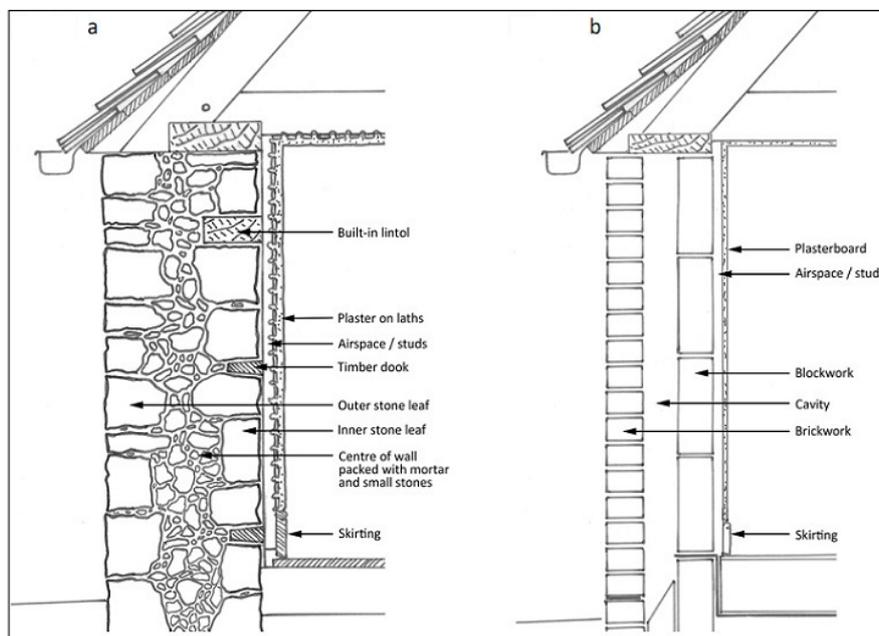
Figure 3. Comparison of (a) traditional solid masonry wall construction and (b) non-traditional cavity wall construction [10].
