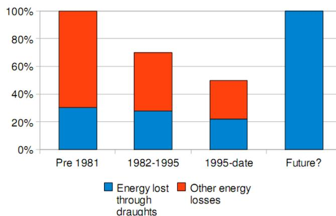
Figure 1. Heat losses [7, 8].
