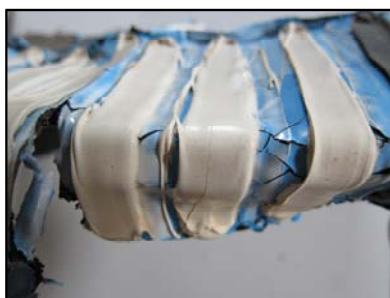
Silicone Polymer Resin Blend Sealant after 2 years in Phoenix Desert Outdoor Weathering Site. No cleaning or special preparation of the sealant. Substrate is a common SAF weather barrier membrane.
