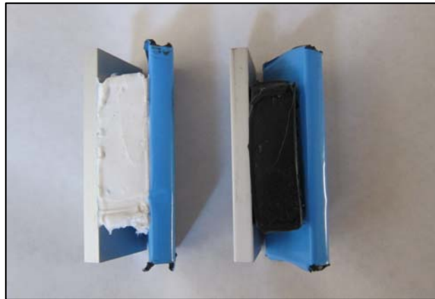
Polymer/resin blend sealant joint after being tested for +/- 25% movement (left) and standard silicone sealant joint after being tested for +/- 25% movement (right). Substrates are anodized aluminum and HDPE.
