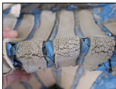
Organic technology sealant after 2 years in Phoenix Desert Outdoor Weathering Site. No cleaning or special preparation of the sealant. Substrate is a common SAF weather barrier membrane.
