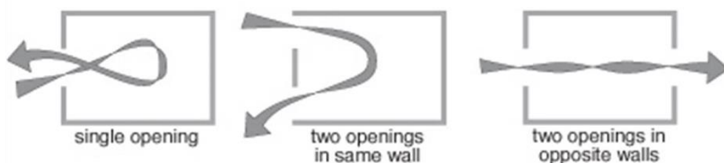
Figure 3: Sectional sketch of Ventilative Cooling Strategies
