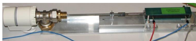
Fig. 3. Experimental set-up for testing electrothermal actuators
