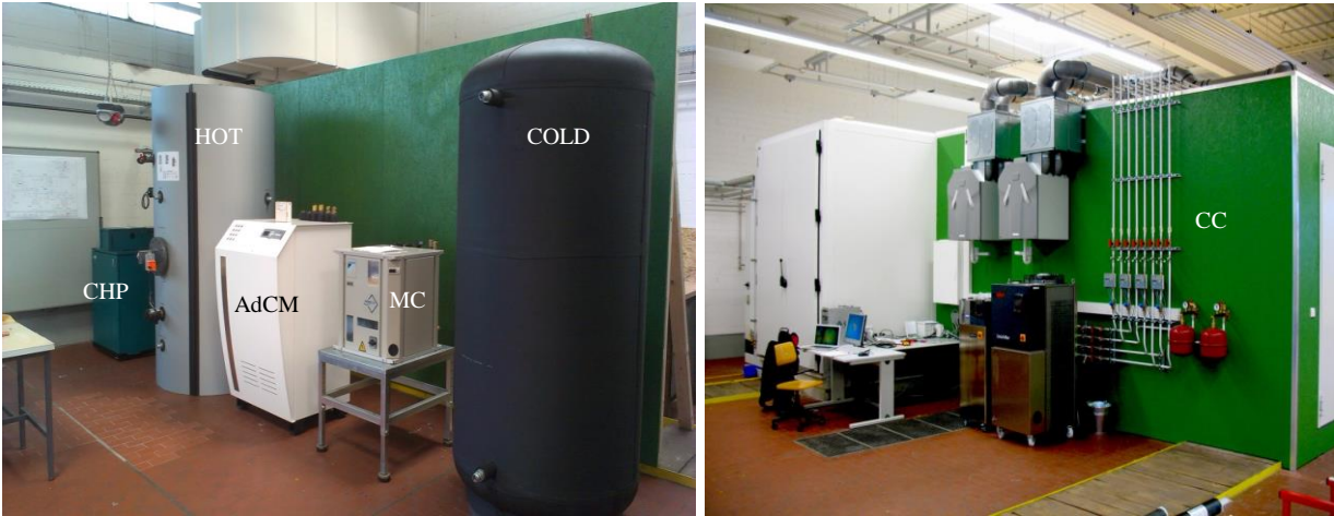
Figure 3: Trigeneration unit and climate chamber (CC) at the Institute of Energy System Technologies (INES)
