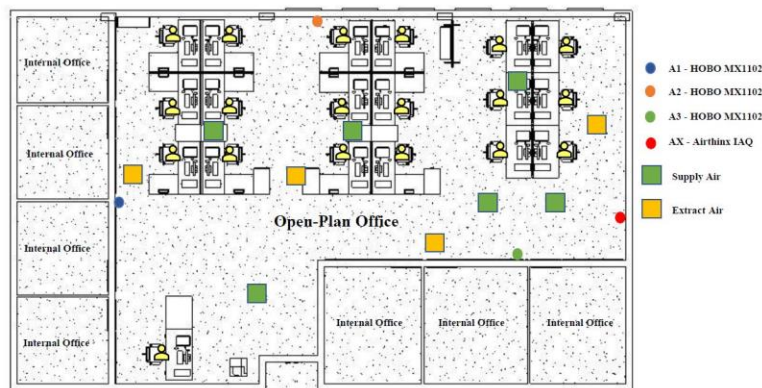
Figure 1 Examined open-plan office layout, including the occupant workplaces, HOBOMX1102 and Airthinx IAQ monitors, and supply and extract air diffusers at the ceiling level.
