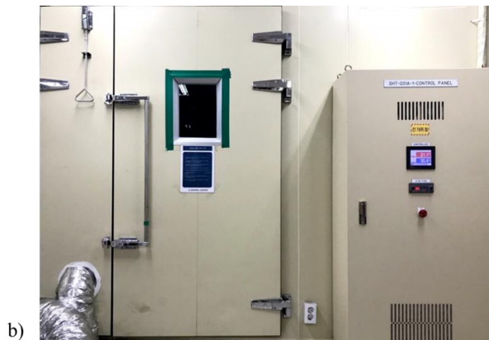
Figure 2 (a) Photo of the HPLD experimental setup (b) Environmental chamber
