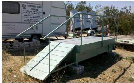
Figure 1: The experimental PV pavement
