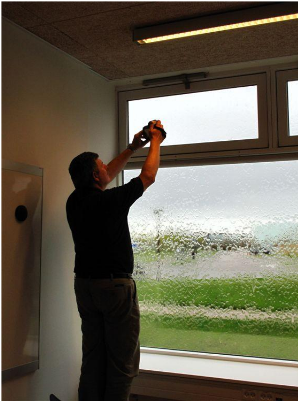
Fig. 3 Window in case 3 undergoing investigating of water penetration with infrared camera
