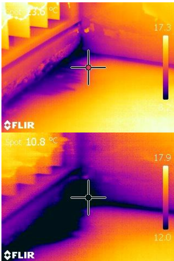
Fig. 1 Example from case 1 of water penetration at 50 Pa at the beginning of the test and after (right)
