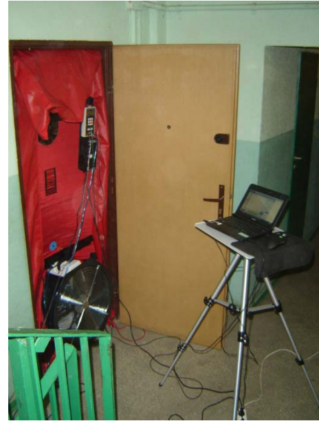
Figure. 1. The test stand for the measurement of the apartment airtightness in multifamily house
