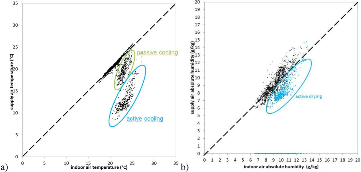
Figure 4: Monitoring results of supply air vs. indoor air: a) temperature, b) absolute humidity.
