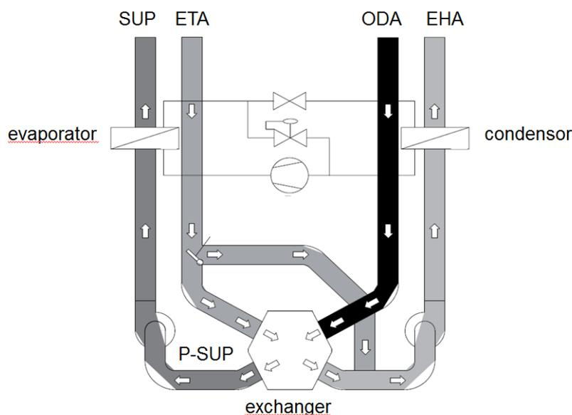
Figure 1: Schematic working principle with outdoor air (ODA), pre-supply air (P-SUP), supply air (SUP, extract air (ETA) and exhaust air (EHA).
