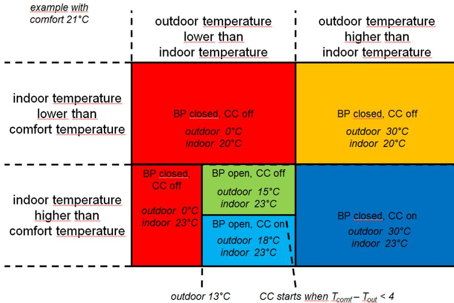
Figure 2: State control diagram
