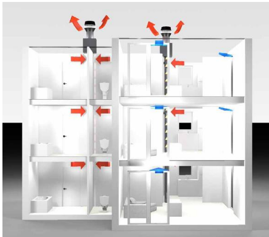
Figure 5: System scheme in hybrid ventilation
