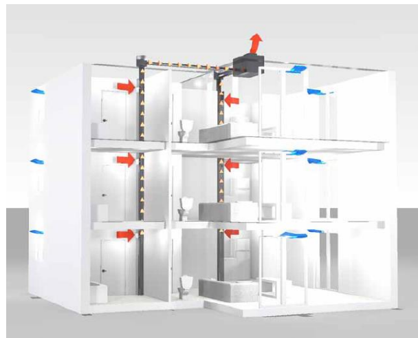
Figure 6: System scheme in mechanical exhaust ventilation (MEV)
