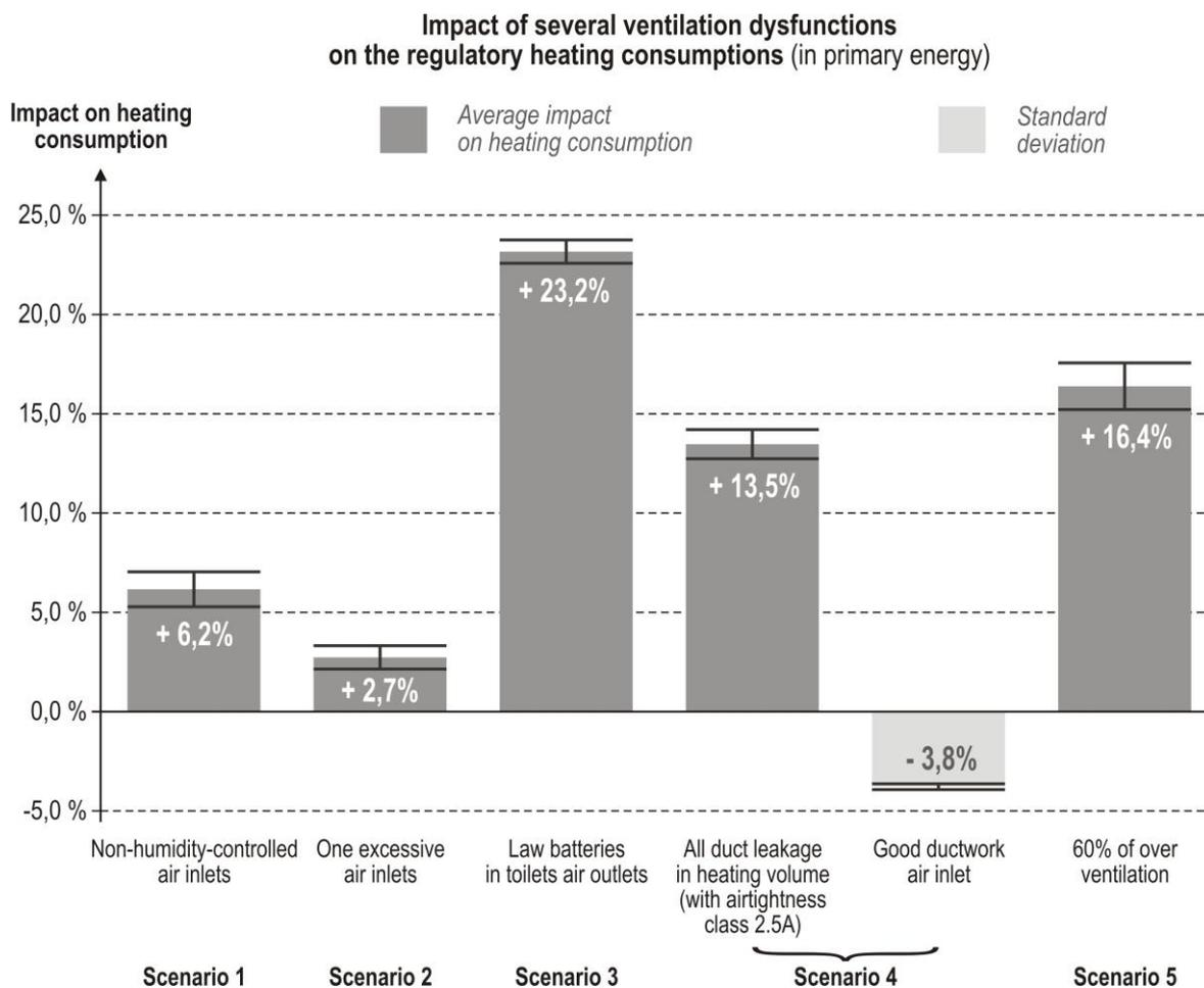
Figure 1: Impact of several ventilation dysfunctions on the regulatory heating consumptions [in primary energy]
