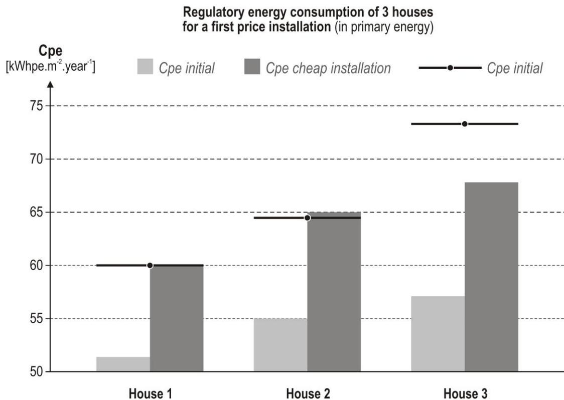
Figure 3: Regulatory energy consumption (primary energy) of 3 houses depending on the ventilation fan performances
