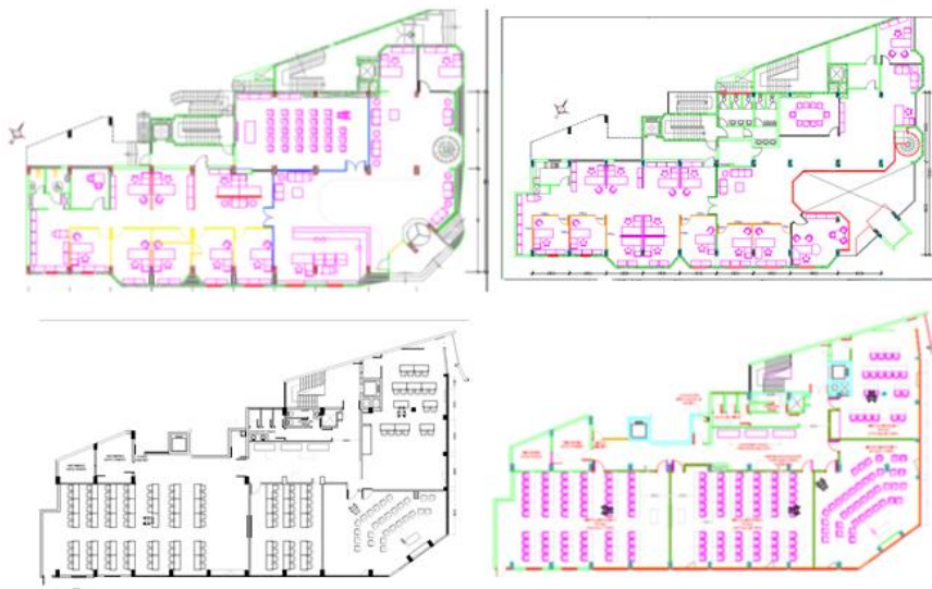
Figure 2: Architectural Design of the building a) Ground floor, b) Mezzanine, c) First Floor, d) Second floor
