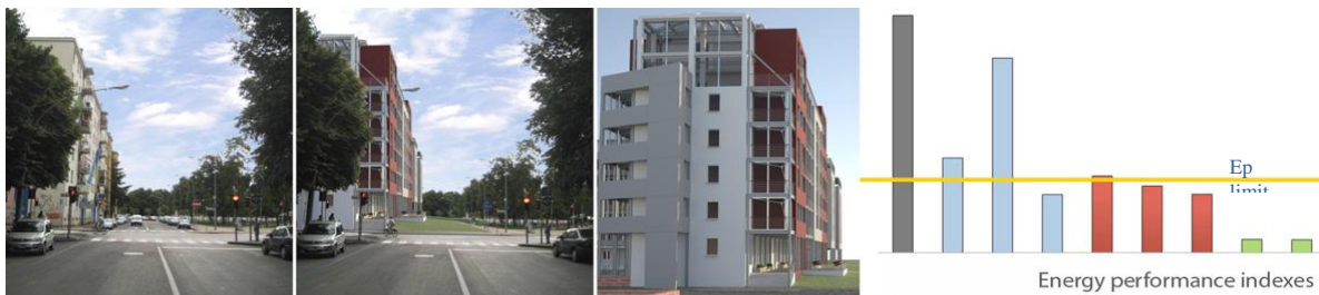
Fig. 1(a, b, c, d). Energy retrofitting by new envelopes design in a reference building of Bologna. a) initial scenario; b,c) new scenario; d) different energy performance indexes ( kWh/m^2 \cdot y ) as a function of different retrofitting options (from left (grey) = initial state; to right (green) = final scenario)
