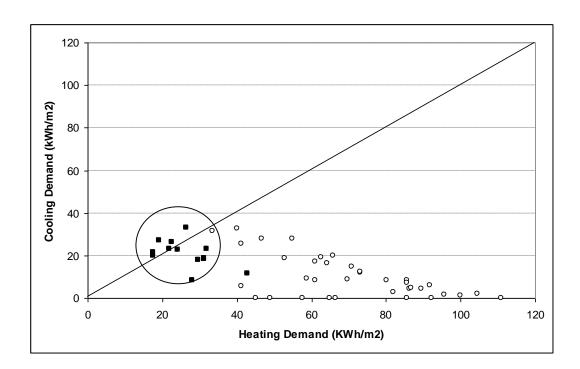
It can be seen that the heating and cooling needs of buildings in locations of Mediterranean climate exhibit a common pattern characterised by low heating needs (compare to other Spanish locations) and relatively high cooling needs often with a ratio cooling/heating close to the unity.
