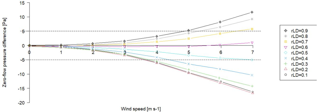
**Figure 4** Experimental zero-flow pressure difference for 9 configurations of leakage distribution depending on wind speed.
