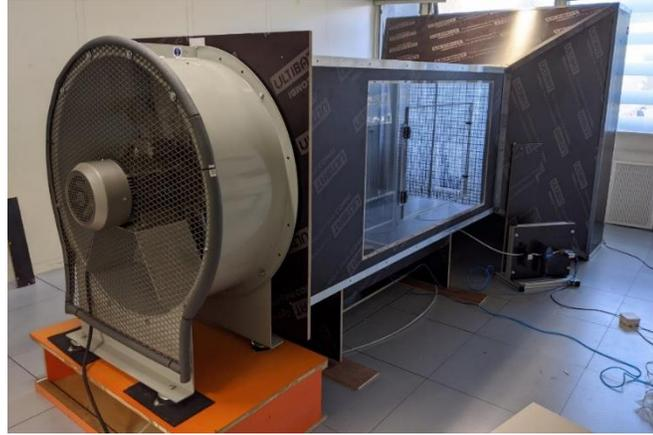
Thanks to our new experimental facility, we performed 96 pressurizations tests based on the ISO 9972 protocol, that include 864 measurements under steady wind conditions: for the nine configurations of leakage distribution of our model and under eight different wind speeds (from 0 to 7 m s<sup>-1</sup> with a step of 1 m s<sup>-1</sup>). In the next section, we analyze the zero-flow pressure differences as it is considered as an indicator of the environmental conditions.
