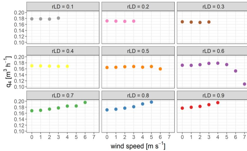
**Figure 4** Variation of  $q_4$  values measured according to ISO 9972 depending on wind speed and leak distribution.
