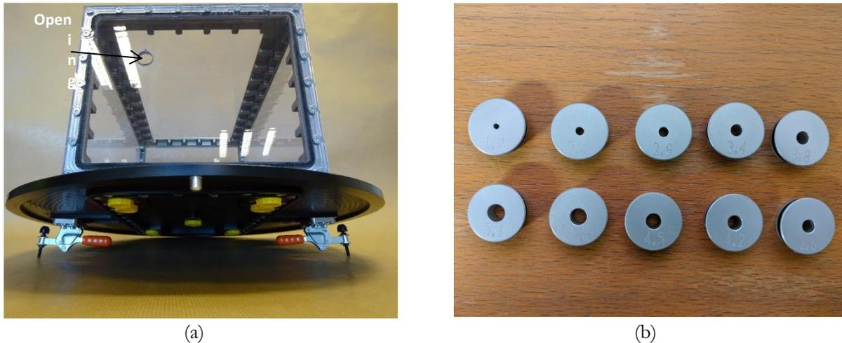
**Figure 1** (a) Final reduced model and (b) Metallic disks with openings corresponding to different  $r_{LD}$  values..
