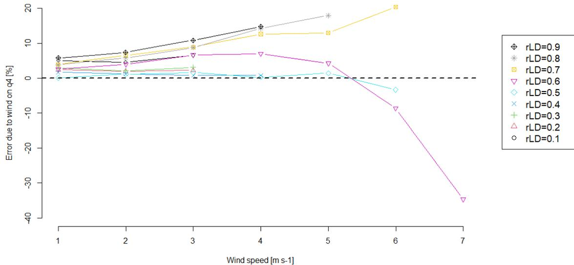
**Figure 5** Error due to wind on  $q_4$  for tests performed according to ISO 9972
