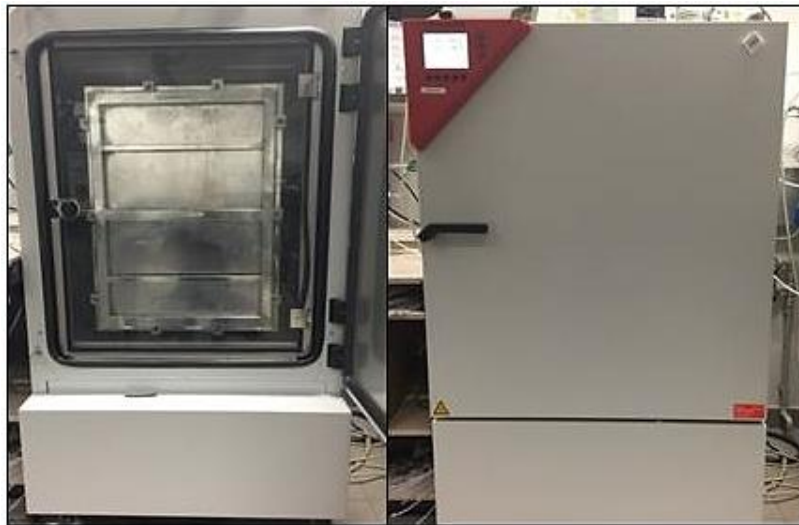
Figure 2 Climate chamber used for source design testing.
