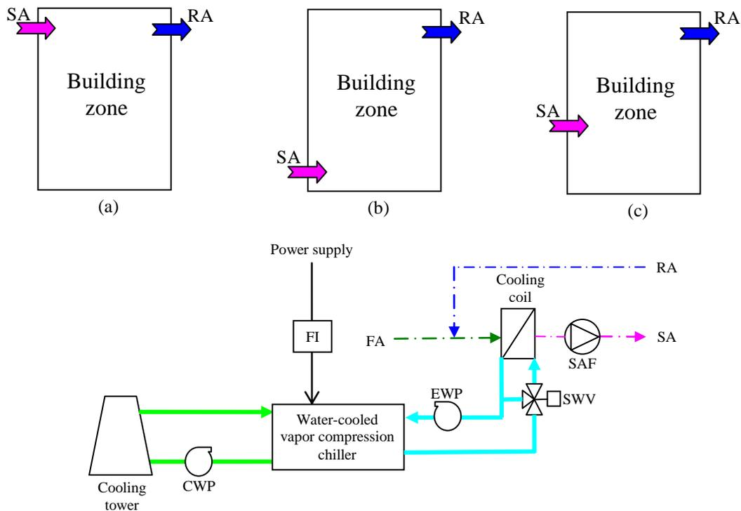
Figure 1 Schematic diagrams of (a) mixing ventilation, (b) displacement ventilation and (c) stratum ventilation systems equipped with an air-handling unit and a variable-speed water-cooled vapor compression chiller
