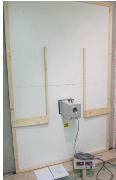
Figure 2: Experimental setup for measurement of the flow resistance
