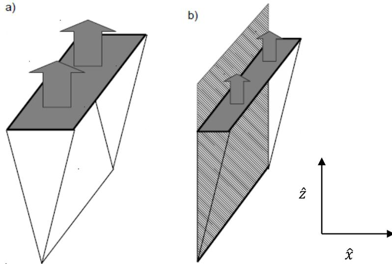
Figure 1: Time-averaged diagram of a free-line plume and a b) wall plume within an environment of constant density.
