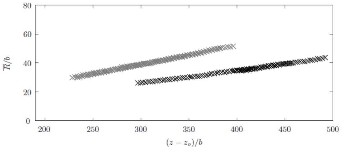
Figure 3: Mean plume widths as defined in (7) for free-line plumes, grey, and wall plumes, black. Both the free-line and wall plume data are scaled on the free-line source width,  $b$ .
