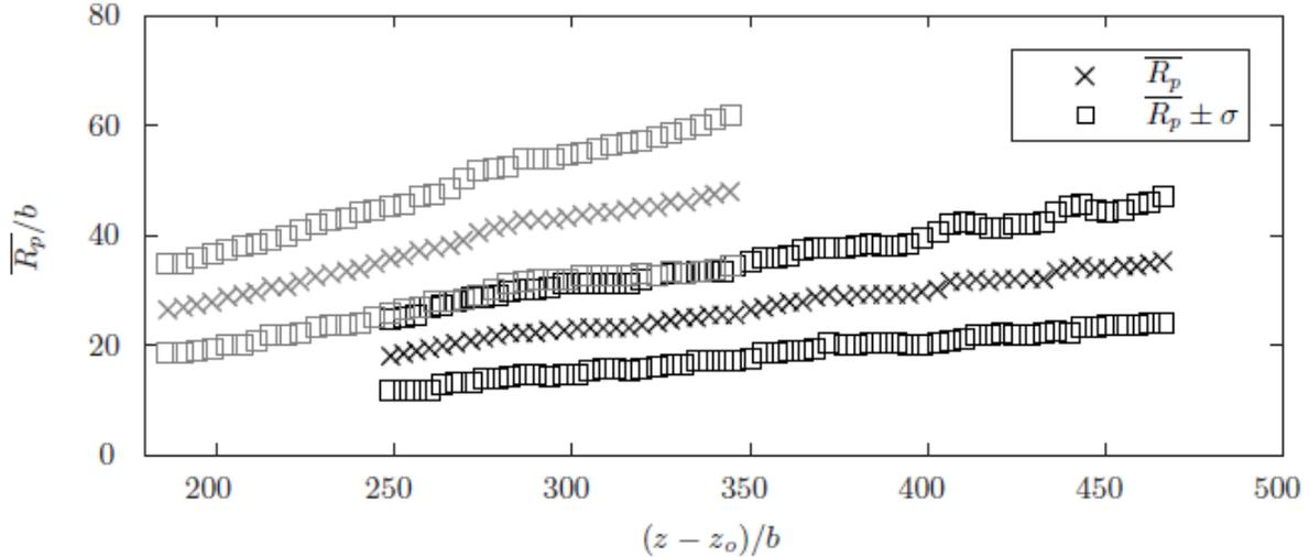
Figure 4: Mean scalar plume widths  $\overline{R_p}$ , crosses, and the variation in scalar plume widths  $R_p \pm \sigma$ , squares, for free-line plumes, grey, and wall plumes, black. Both the free-line and wall plume data are scaled on the free-line source width,  $b$ .
