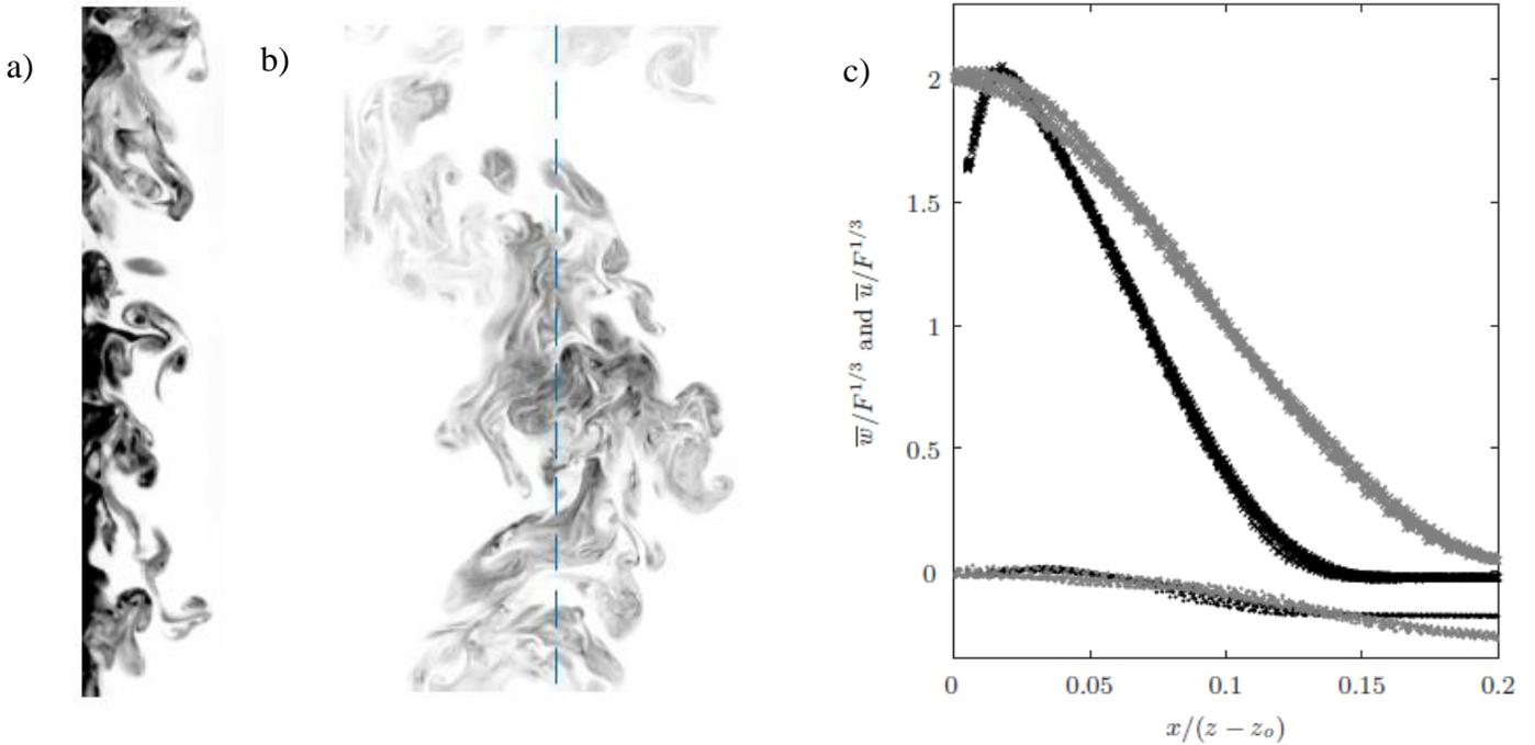
Figure 2: A snapshot of the experiment for a) a wall plume and b) free-line plume. The blue dashed line indicates the position of the source. c) Vertical, crosses, and horizontal, dots, velocity data for free-line, grey, and wall plume, black. Data from experiments 1 are used in both cases and 20 heights are plotted spanning the whole height. For the wall plume case the velocities are scaled using double the physical buoyancy flux in order to make a direct comparison of the velocities.
