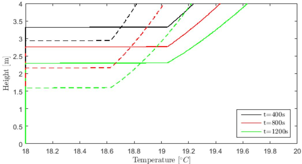
Figure 5: Evolution of the ambient temperature stratification profiles of free-line plume (dashed lines) and wall plumes (solid lines) for times  $t=400s$  (Black),  $t=800s$  (Red) and  $t=1200s$  (Green).
