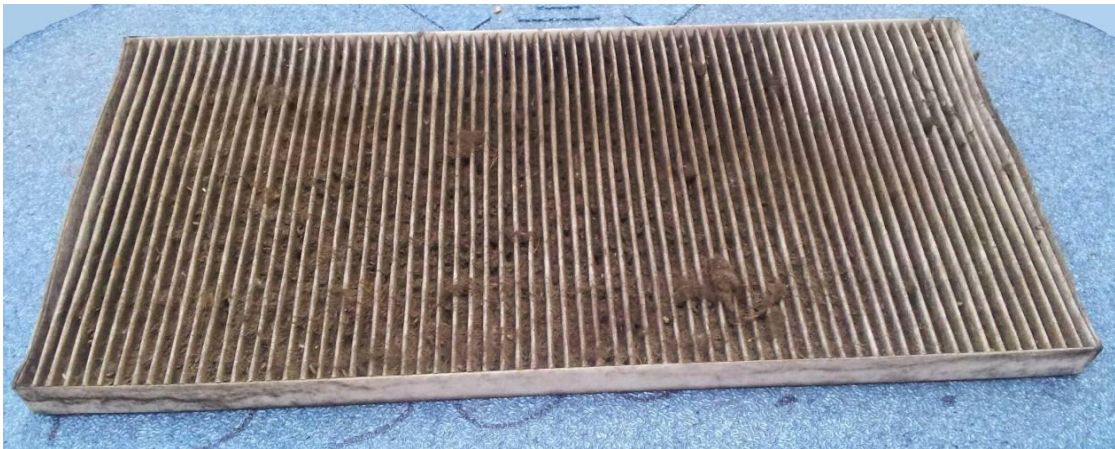
Figure 13 : Filter E after 1 year of use (pleat width 6.1 mm)
