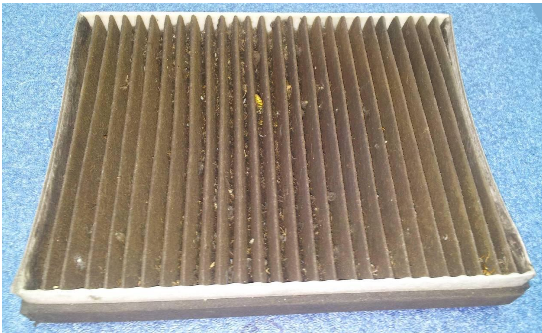
Figure 14 : Filter F after 1 year of use (pleat width 10.4 mm)
