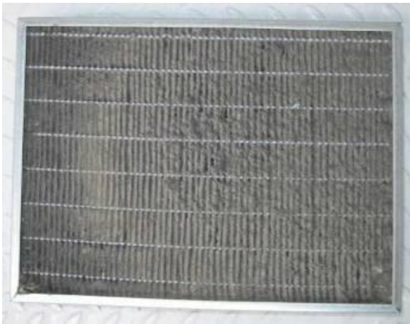
Figure 9 : Filter C not protected by a prefilter, after 1 year of use
