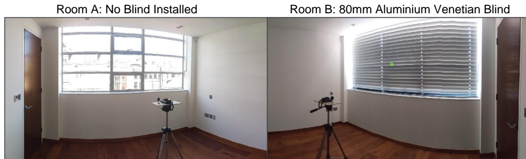
Figure 3. Room A and B in Unit 18 with sensor setup.
