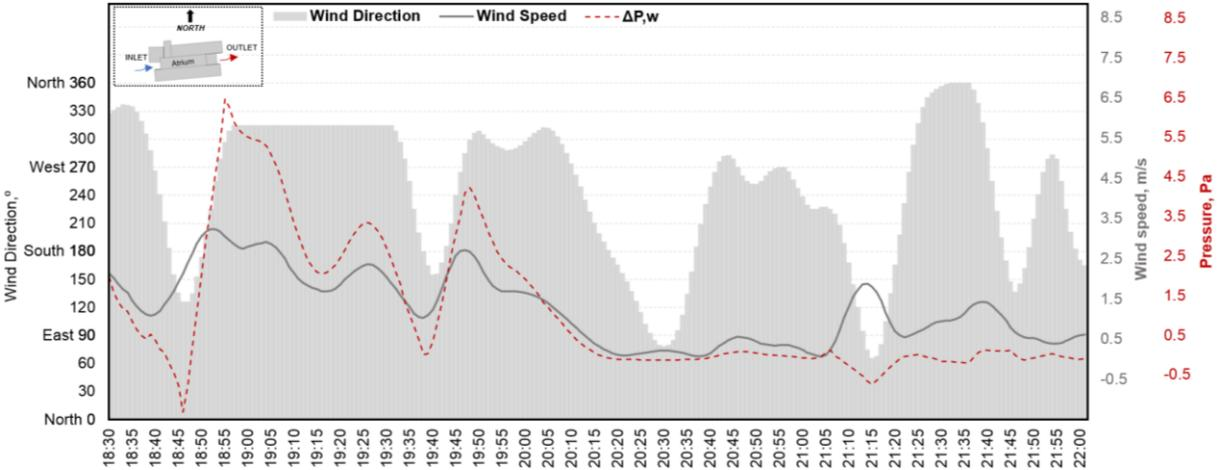
Figure 3 Wind distribution, wind speed and pressure generated by the wind
