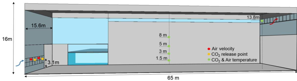
Figure 2 Location of the sensors used for the experiment and CO<sub>2</sub> release point location
