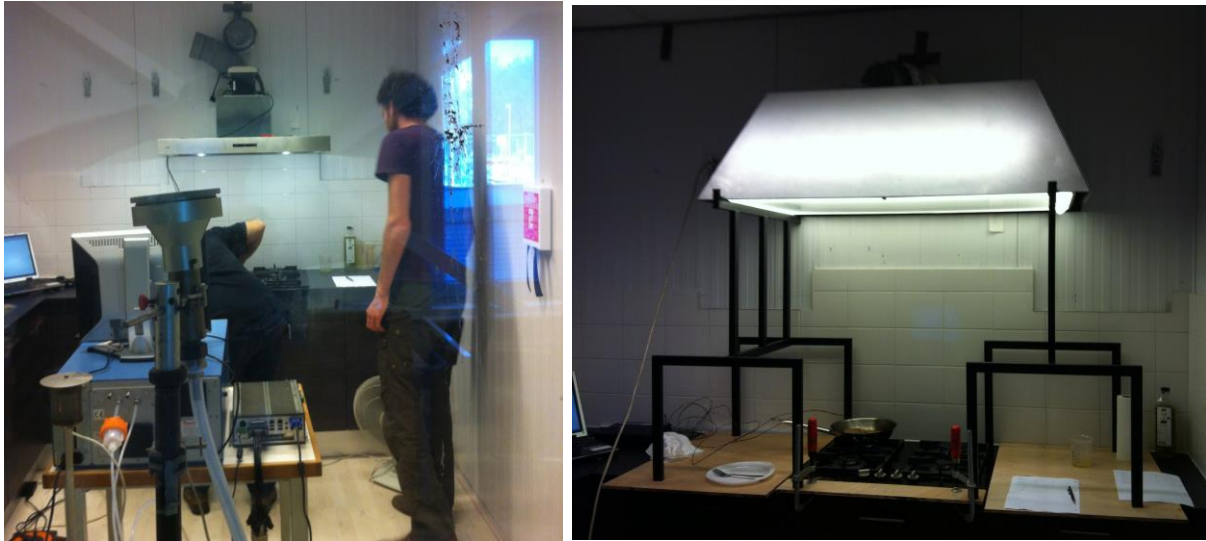
Figure 2: left positioning of recirculation hood and measurement equipment, right plasma hood.
