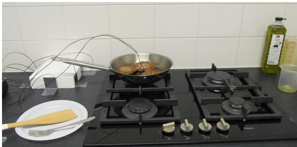
Figure 1: frying hamburgers in stainless steel pan with temperature sensor.
