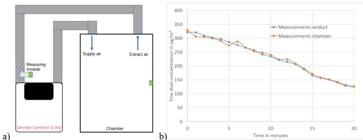
Figure 3: a) Experimental set-up of validation measurement for the PM sensor prototype and b) measured PM<sub>2.5</sub> values (sensor values in test chamber in orange and PM sensor prototype values in blue)
