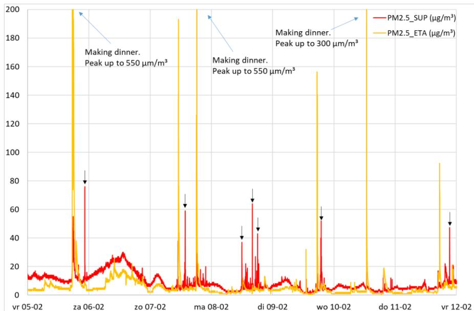
Figure 6: PM<sub>2.5</sub> values in extract air (yellow) and in supply air (red) in Lettele.
