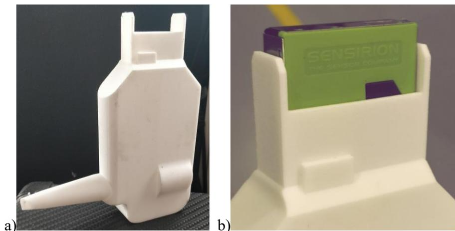
Figure 2: a) 3D printed PM sensor prototype, b) close-up of upper part of the prototype with the green PM sensor component inserted
