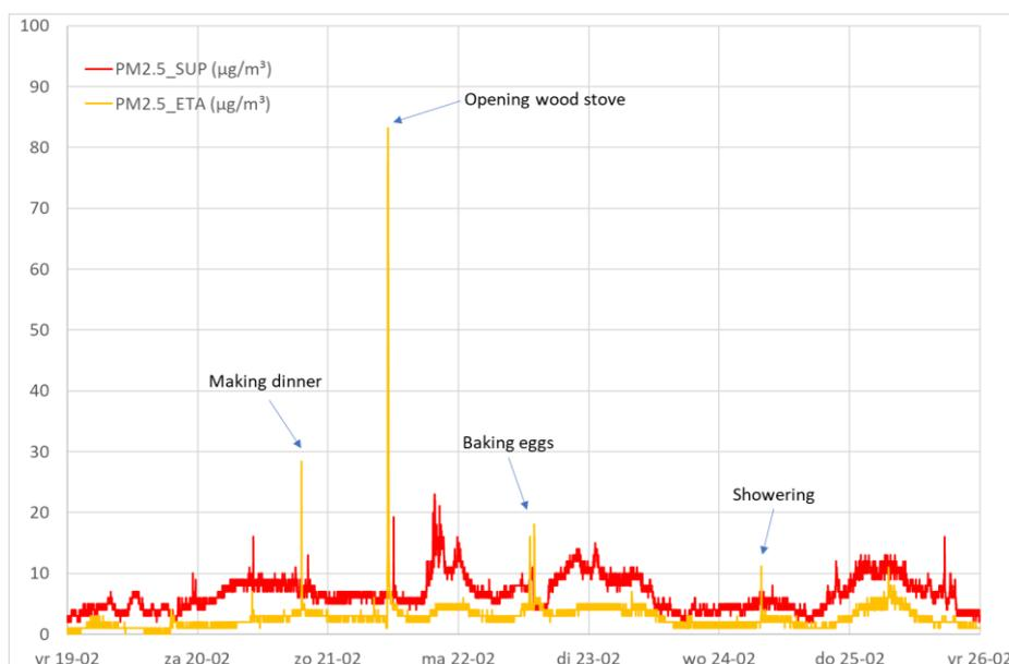
Figure 7: PM<sub>2.5</sub> values in extract air (yellow) and in supply air (red) in Zwartsluis.
