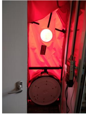
Figure 7 - Kitchen (side) door has potential interference from internal doors.
