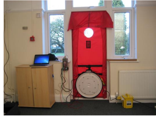
Figure 8 – Blower door apparatus set up in the rear door (dining room). All main tests were conducted from this opening.
