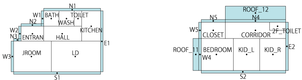
Figure 2: Zones and airnodes of the building model in TRNSYS
