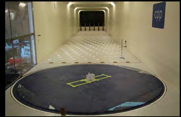
Sealed model at 1:100 scale with 299 pressure taps spread over 5 facades
