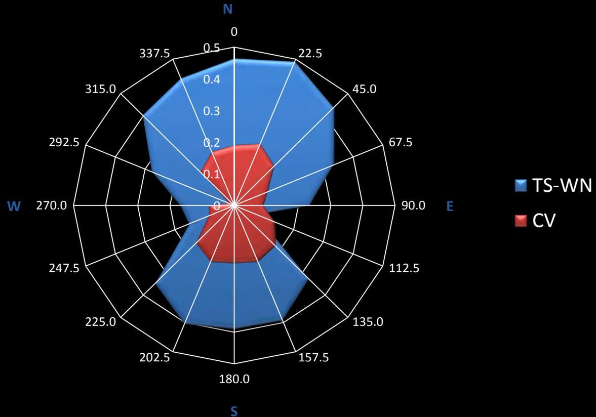
Mean indoor air speed in Jan 2013 via wind tower south opening & north window (TS-WN)
