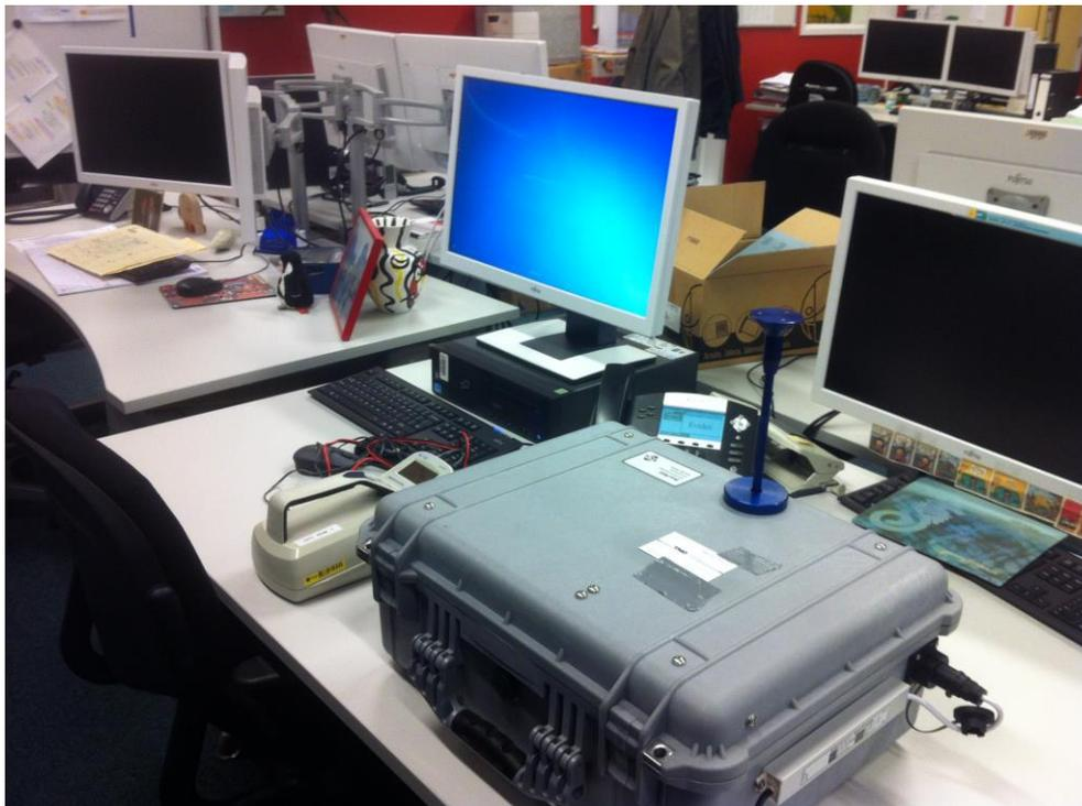
Figure 1: optical particle counter placed in suitcase in an office room.
