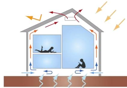
Figure 1: Double-skin system of room-side air gap applied to detached house
