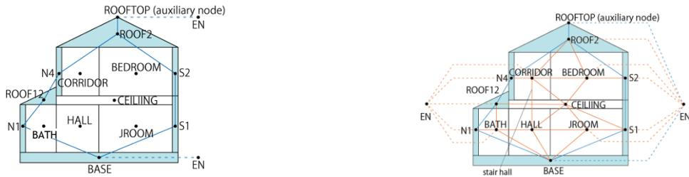
Figure 5: Overview of air links (simple model)
