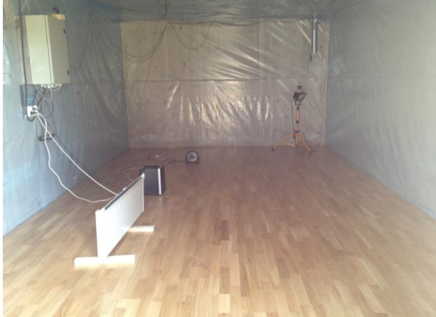
Figure 2: Interior view of module B where the walls and ceiling are upholstered in PE foil.
