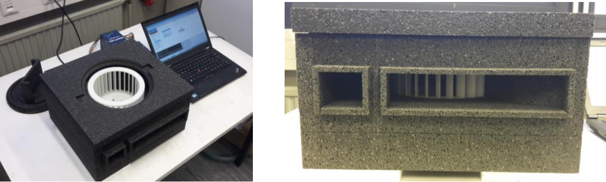
Figure 9. Photo of the manufactured laboratory prototype of the CHRF for the use as single/double room unit.
