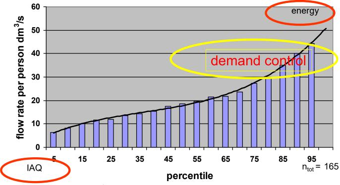
No person has a mean air flow rate over the heating season lower than 4.9 dm3/s
