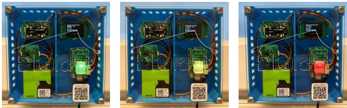
Figure 2: Example of the feedback colours at three different CO 2 levels of the used device
