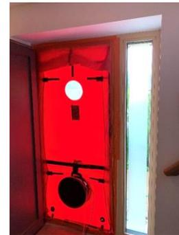
Figure 4: Blower door fan setup in a doorway and taped from inside
