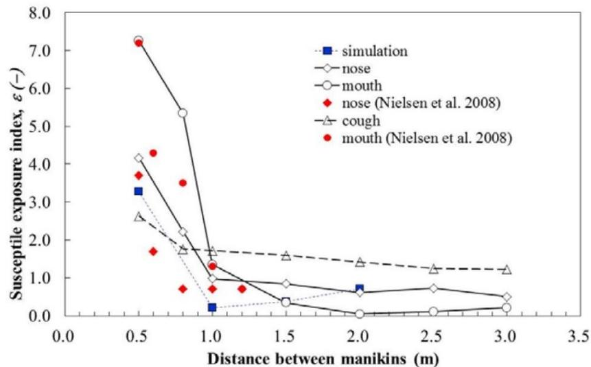
Figure 6. Exposure of target manikin versus distance between the two manikins of same height in a room with displacement ventilation. Results are shown for both breathing through the mouth, through the nose, for coughing and for CFD predictions (Liu et al. 2017).
