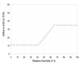
Figure 6: Airflow as a function of relative indoor humidity in a humidity controlled air terminal (e.g. air inlet)
