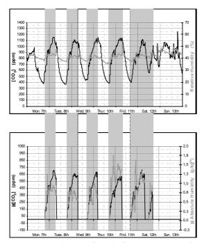
Figure 4: CO<sub>2</sub> and H<sub>2</sub>O changes in a single room. Top: continuous measurements of CO<sub>2</sub> and relative humidity. Bottom: measurement of *CO*<sup>2</sup> and absolute humidity during occupied periods only (nights)
