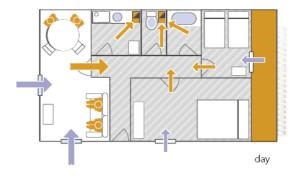
Figure 10: Typical day-time dispatching of airflows within the dwelling
