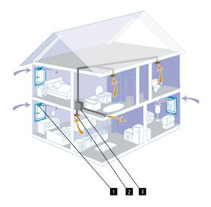
Figure 9: Airflows and humidity sensitive components in a single-house mechanical ventilation system.
