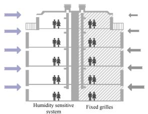
Figure 13: Humidity control of ventilation balances the airflows across floors in passive stack ventilation
