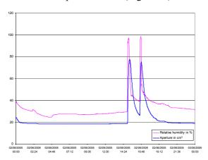
Figure 14: Opening of the humidity sensitive air extract grille (blue, in cm²) and indoor relative humidity (pink, in %) over one day, in a bathroom.
