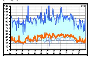
Figure 15: Range and mean daily airflows in a bathroom over one year. Blue: minimum and maximum airflows. Red: mean airflow.
