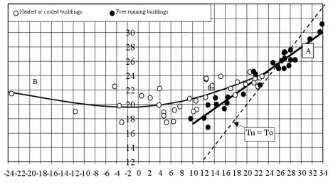
Figure 3: The change in comfort temperature with monthly mean outdoor temperature for free floating and air conditioning buildings, (From Nicols 2003)
