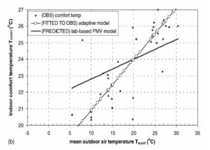
Figure 1: Observed (OBS) and predicted indoor comfort temperatures from RP-884 database, for naturally ventilated buildings, (from De Dear and Brager 2002)
