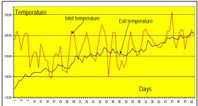
Figure 10: Inlet and outlet temperatures in one of the heat exchangers during the summer period
