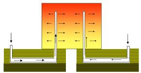
Figure 1: Principle of earth to air heat exchangers
