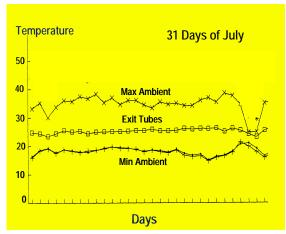
Figure 7: Performance of earth to air heat exchangers at the University of Ioannina
