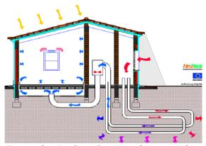
Figure 2: A close loop earth to air heat exchanger [Ref. 1]
