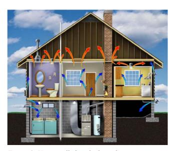
Figure 1: Uncontrolled air leakage, known as air infiltration, across the building envelope of a house. <sup>1</sup>
