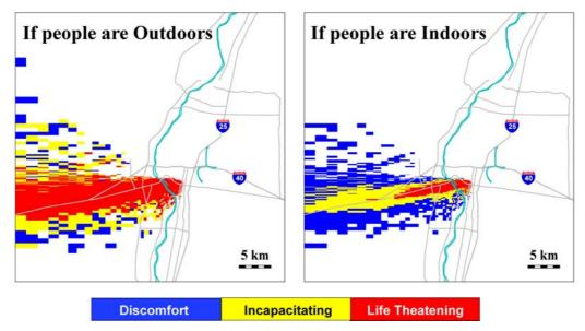
Figure 6: Predicted health effects based on US EPA's Acute Exposure Guidelines [24] of a hypothetical 4-hour chlorine gas release in Albuquerque if shelter-in-place is implemented (right) compared to if everyone is outdoors (left).
