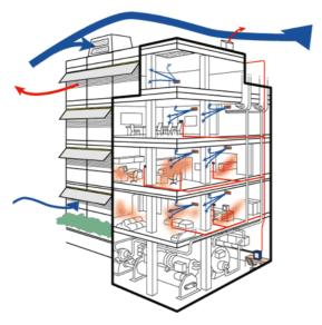
Figure 4: Commercial buildings can have complicated airflow pathways; contaminant concentrations may be non-uniform for a long time.
