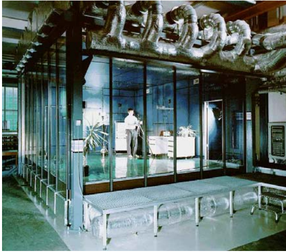
Figure 6.1: Room climate laboratory at EMPA, Test room dimensions: 6.2 \times 4.6 \times 3.0 \text{ m}^3
