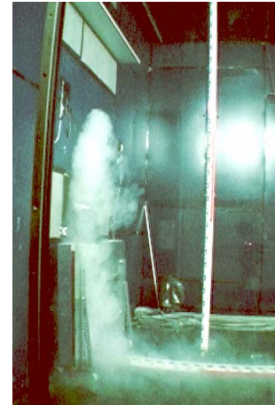
Figure 6.4: The penetration depth of the discomfort zone in the below position is less than in the above position, whereas the draft risk along the floor is remarkably high - Floor heating.
