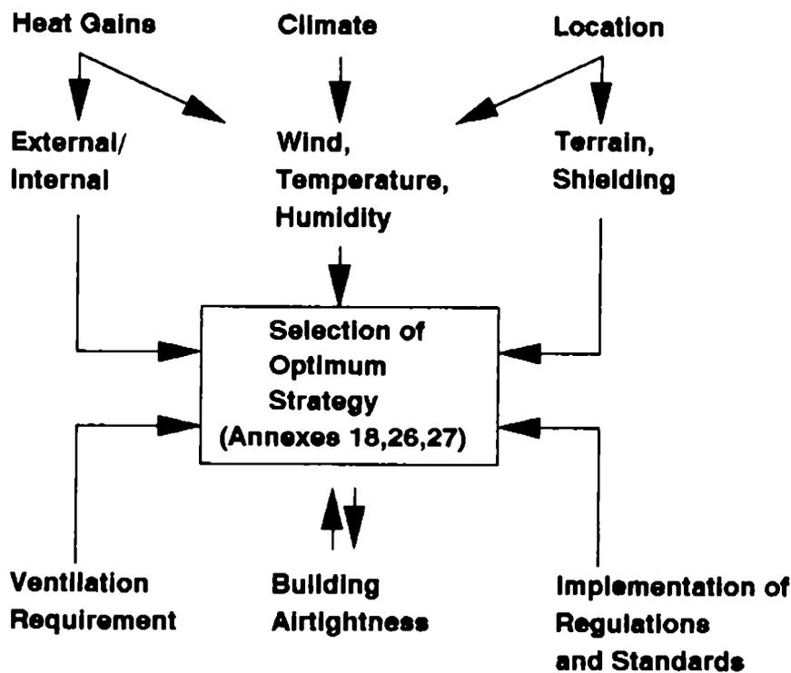
Figure 8: Achieve energy and cost effective ventilation - design tools
