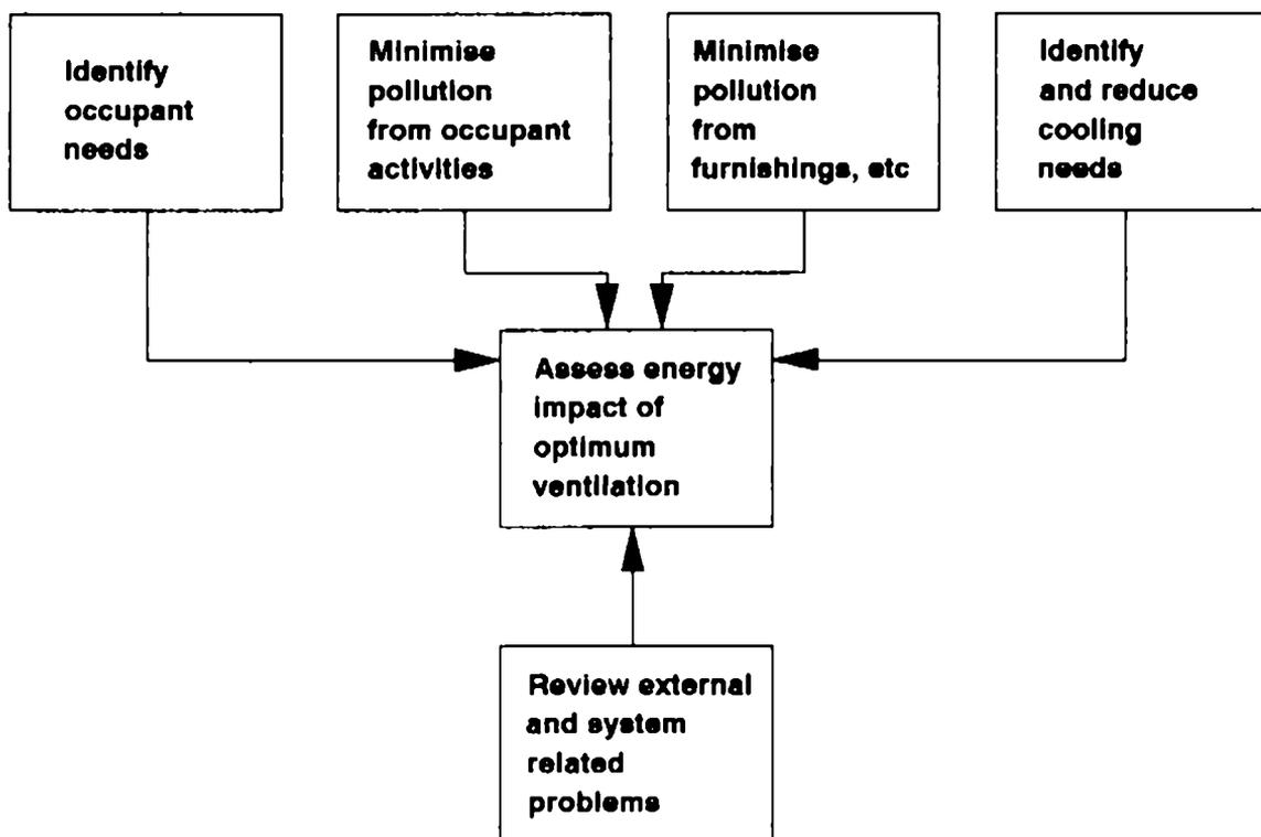
Figure 5: Optimum ventilation needs
