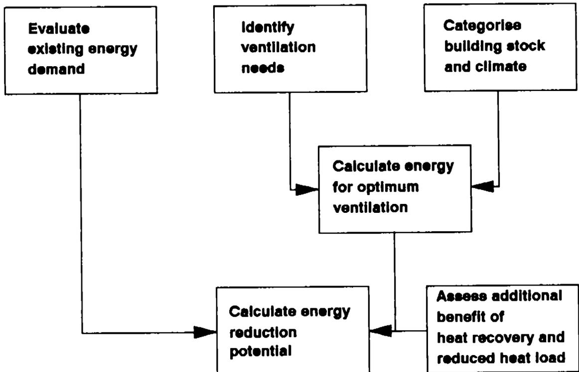
*Figure 6: Achieve energy and cost effective ventilation - system design needs*
