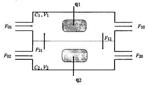
Fig. 4.1 Schematic diagram of a two zone model.
