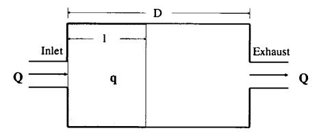
Fig. 3.6 Piston Flow - Uniform Injection between the Inlet duct and a Plane across the Room.
