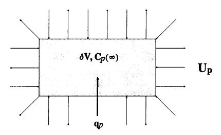
Fig. 2.1 Illustration of the local purging flow rate.
