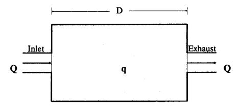
Fig. 3.2 Piston Flow - Uniform Injection Throughout the Whole Space
