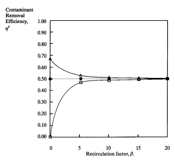
Figure 4.3 - Contaminant removal efficiency vs recirculation factor.
