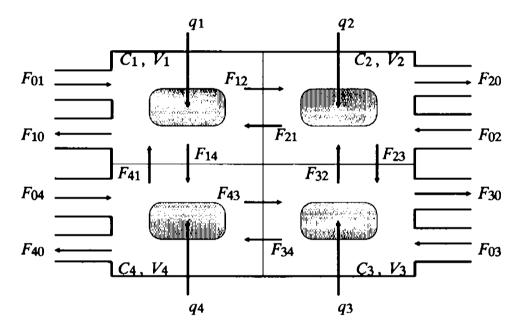
Fig. 5.1 Schematic Diagram of a 4 Zone Model
