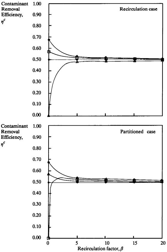
Figure 5.3 - Contaminant Removal Efficiency vs recirculation factor.
