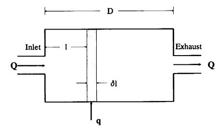
Fig. 3.4 Piston Flow - Localised Injection in a Plane across the Room.
