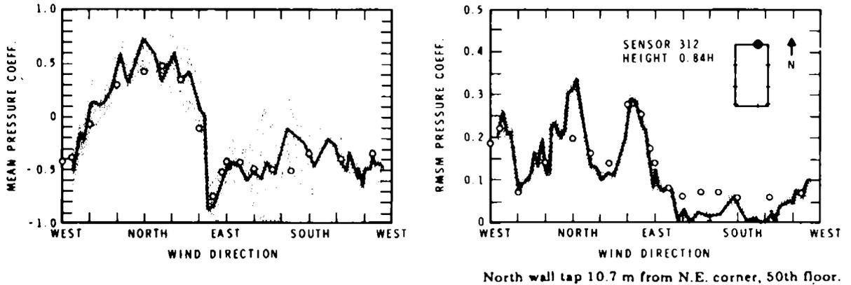
Fig. 14. Example of full scale measurements on a 57 storey office tower in Toronto. (from Dalgliesh<sup>10</sup>)
