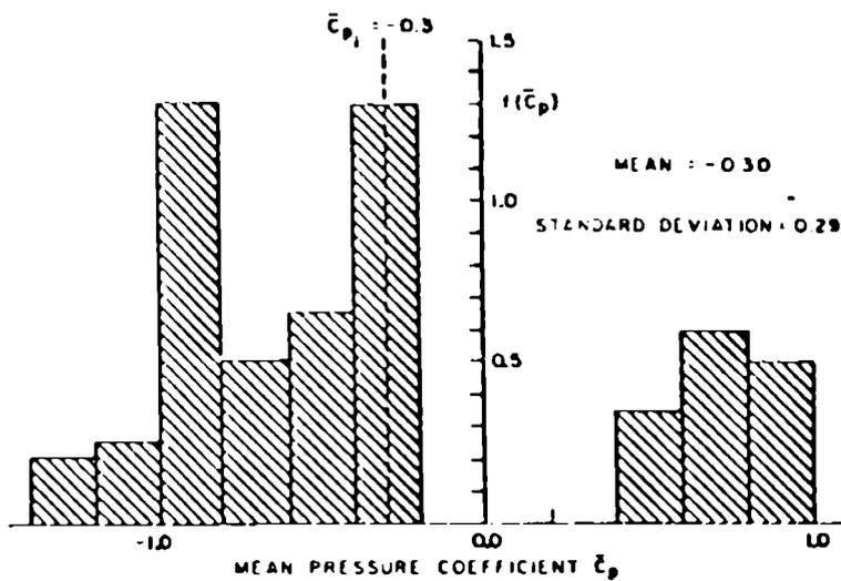
**FIG. 2 DISTRIBUTION OF TIME AVERAGED EXTERIOR PRESSURE COEFFICIENTS ON A TALL BUILDING IN BOUNDARY LAYER FLOW REFERENCED TO ROOF HEIGHT**
