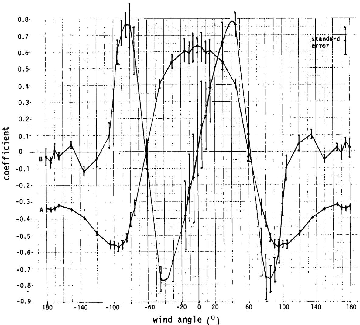
Fig. 5 Fourier analysis of the horizontal pressure distribution across a facade with wind angle. (see eqn. 2) (data from Bowen<sup>3</sup>)
