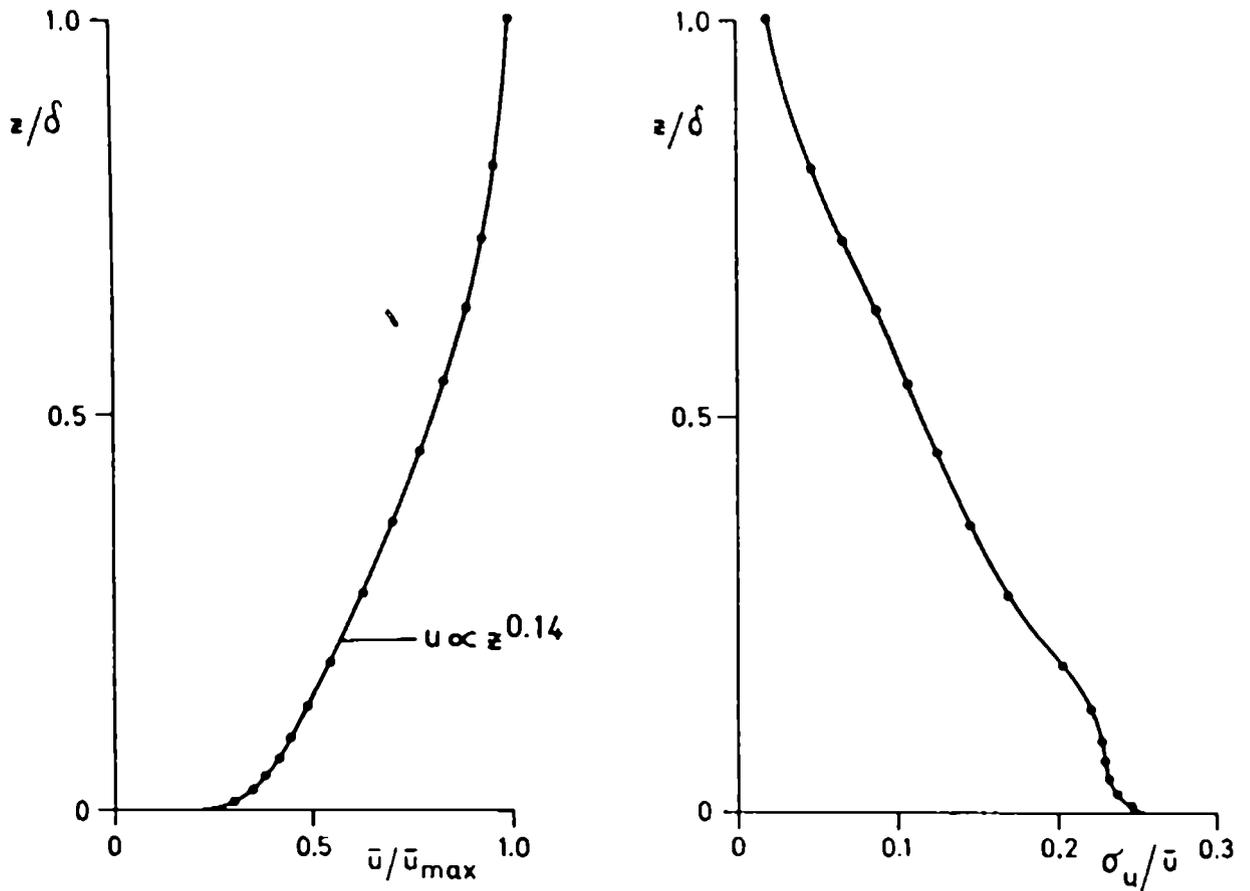
Fig. 2. Mean velocity and turbulence intensity profiles of the model boundary layer flow.
