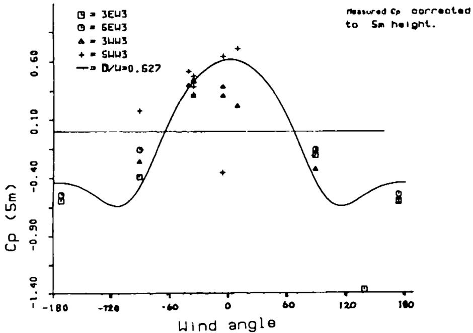
Fig. 12b Measured and calculated pressure coefficients plotted against wind angle for the Aylesbury test house.
