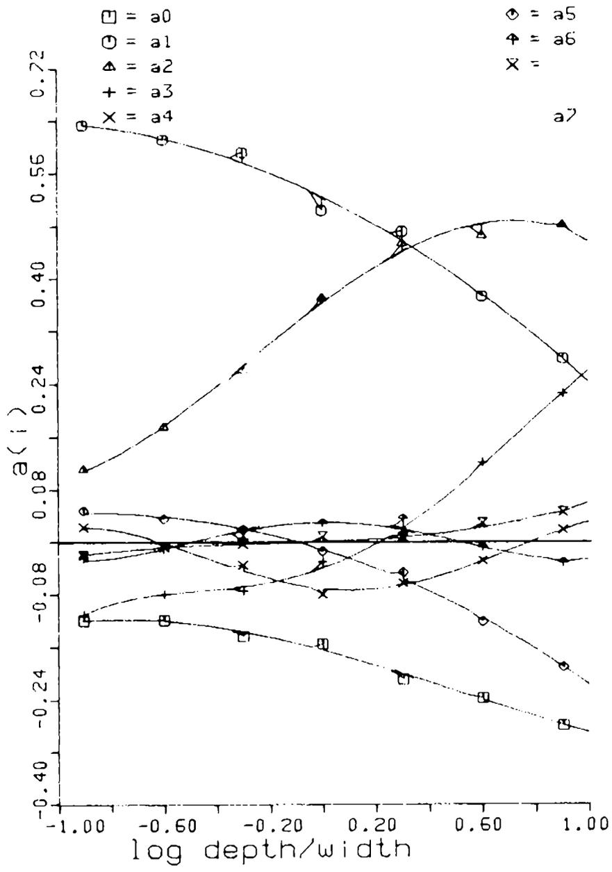
Fig. 2 Coefficients a(i) for roof level pressure coefficients.
