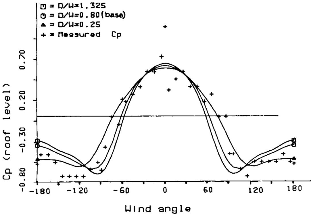
Fig. 8a Measured and calculated pressure coefficients plotted against wind angle for position 6 (side wall).
