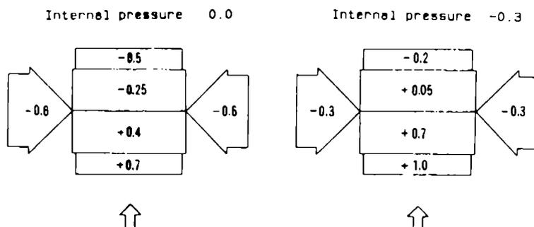
Figure 2 Pressure coefficients from the code of practice
