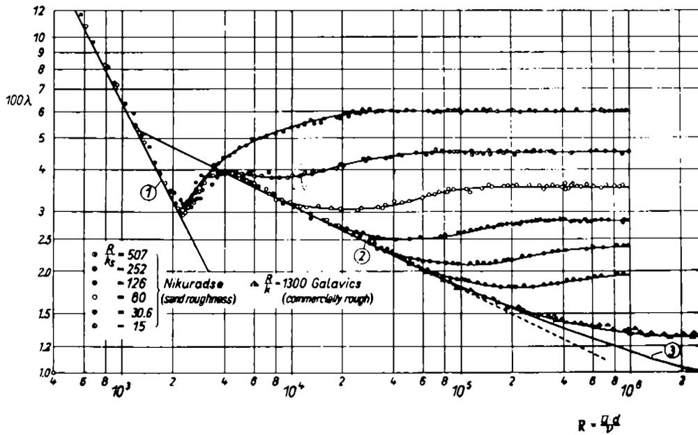
Fig. 1. Frictional resistance, rough pipes.
