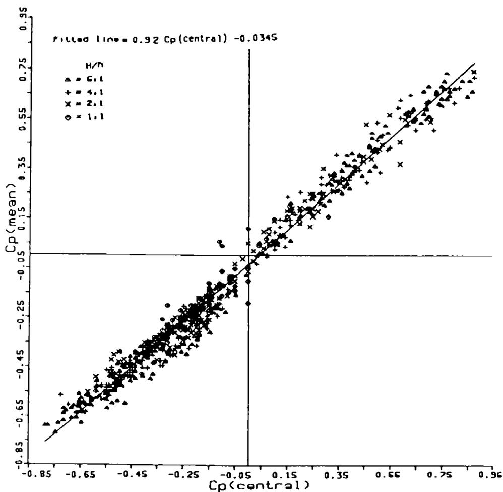
Fig. 9 Plot of mean Cp against centre line Cp for various z/H, H/h and wind angle for face A. (see Fig. 4) (data from Bowen<sup>3</sup>)
