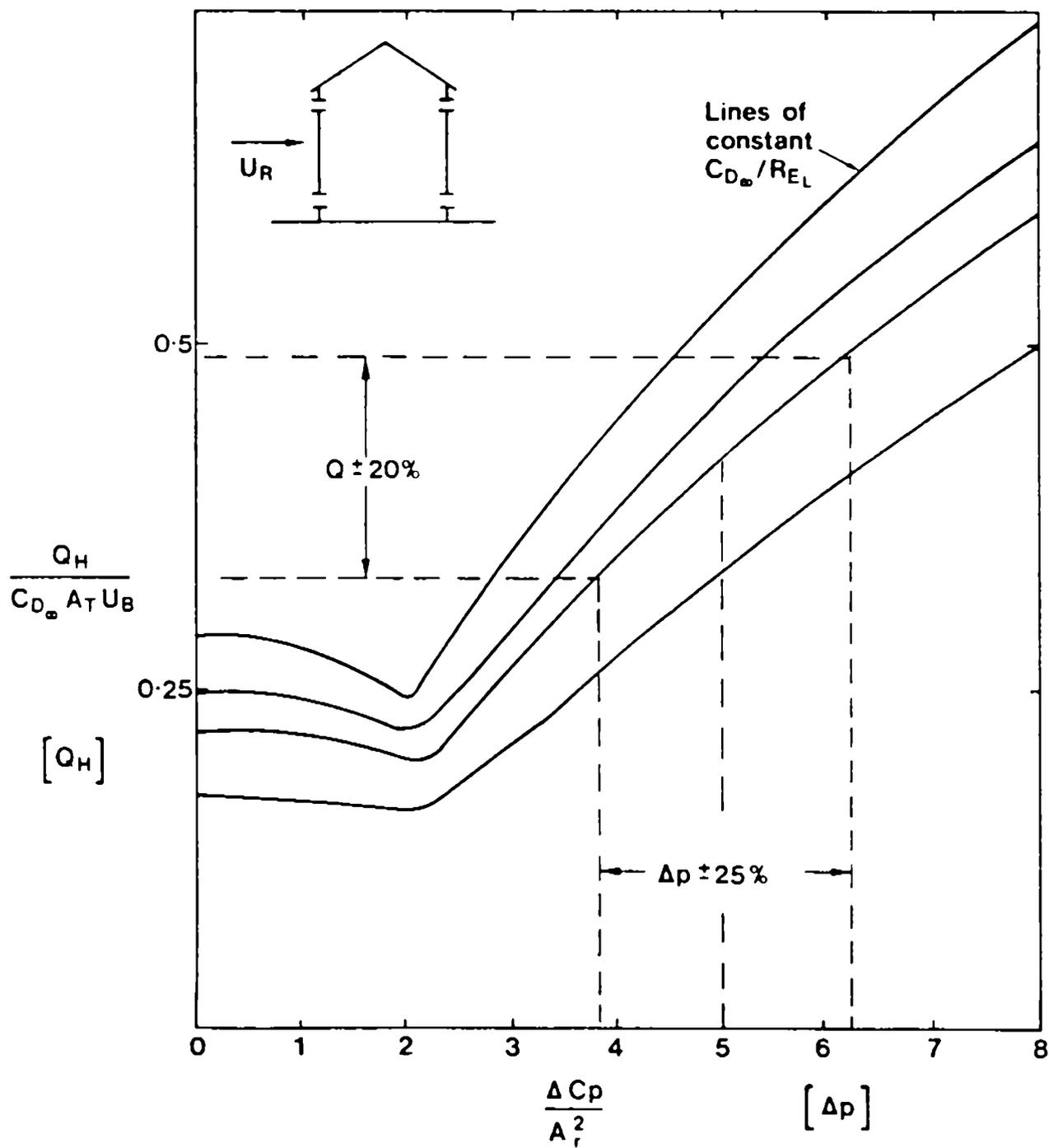
Fig.1 EXAMPLE OF SENSITIVITY OF VENTILATION RATE  $Q_H$  TO PRESSURE DIFFERENCE  $\Delta p$
