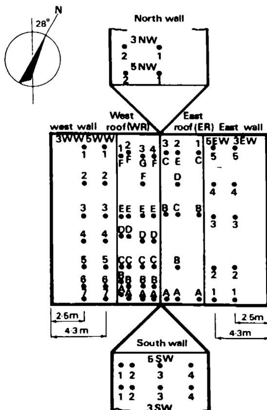
Fig. 11 Aylesbury Test House - location of pressure taps
