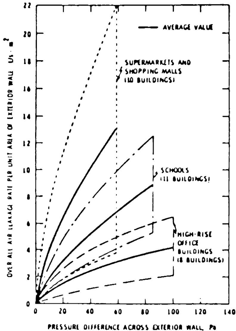
FIG. 1 COMPARISON OF OVERALL AIR LEAKAGE OF VARIOUS BUILDING GROUPS (after Tamura and Shaw - 1981)
