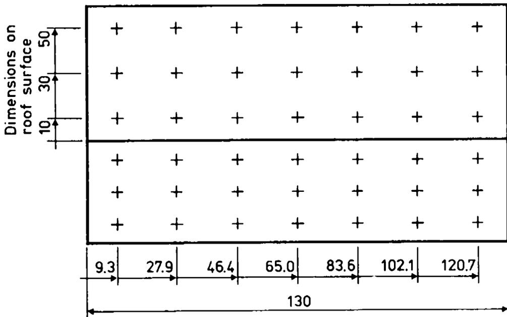
Fig.3 Position of pressure taps on the model
