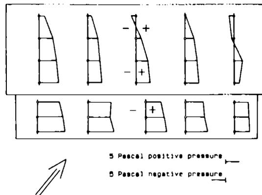
Figure 8 Pressure distribution on the windward wall and roof
