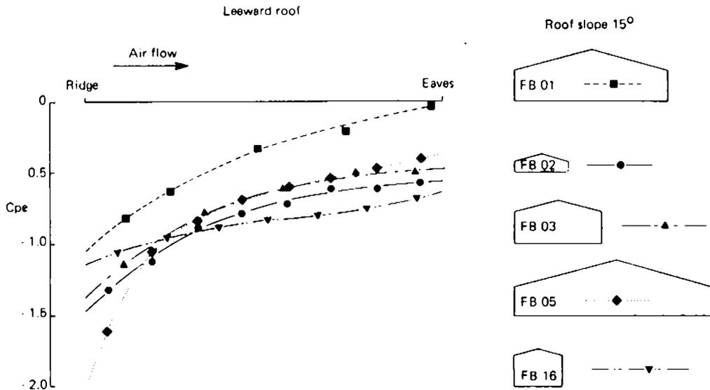
Fig. 2. Pressure distribution on the leeward roof for a selection of buildings with a 15° roof slope
