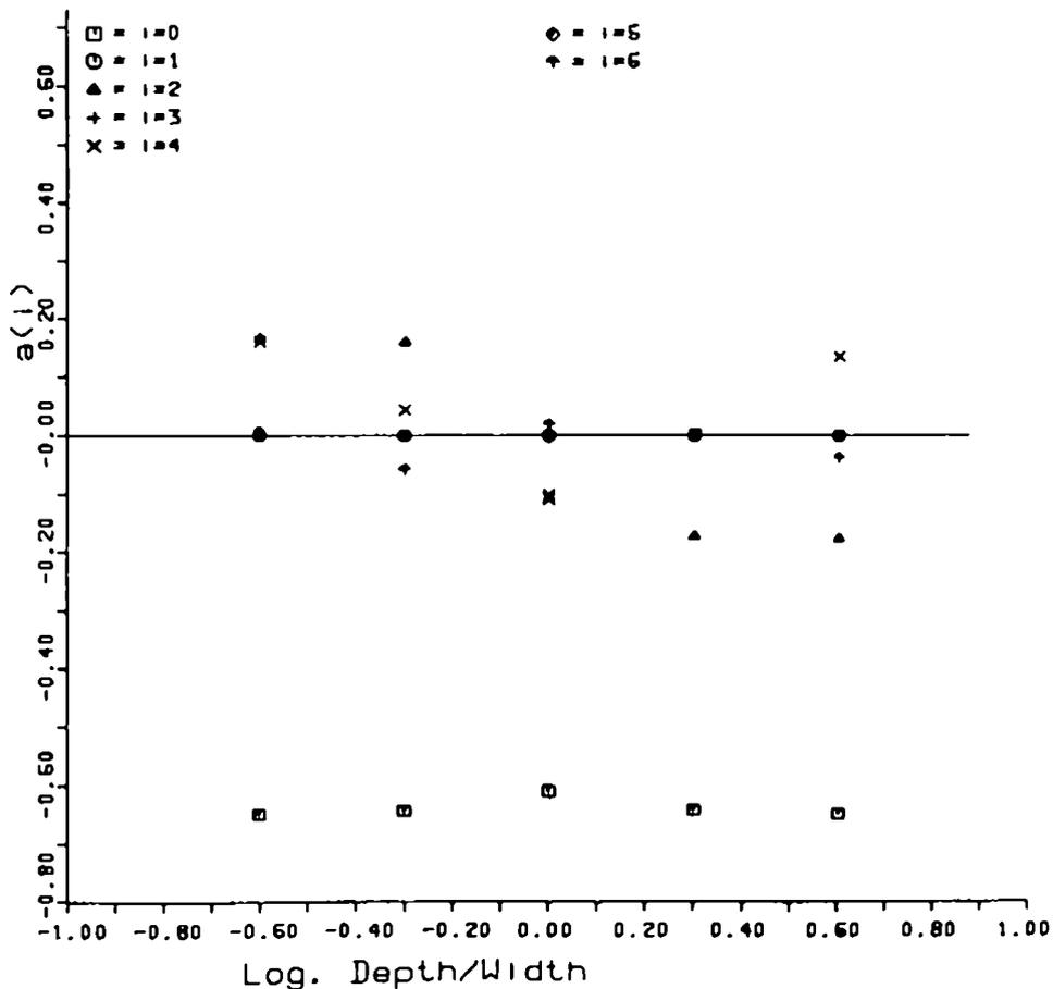
Fig. 6 Coefficients  $a(1)$  from eqn. 7.1 for the mean  $C_p$  of a flat roof. (same for both roof level and local reference winds)
