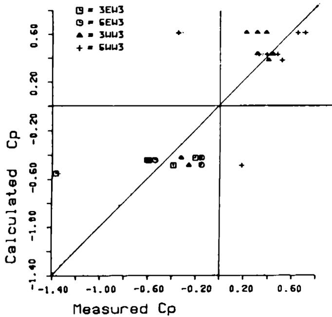
Fig. 12a Measured vs. calculated pressure coefficients for the Aylesbury test house.
