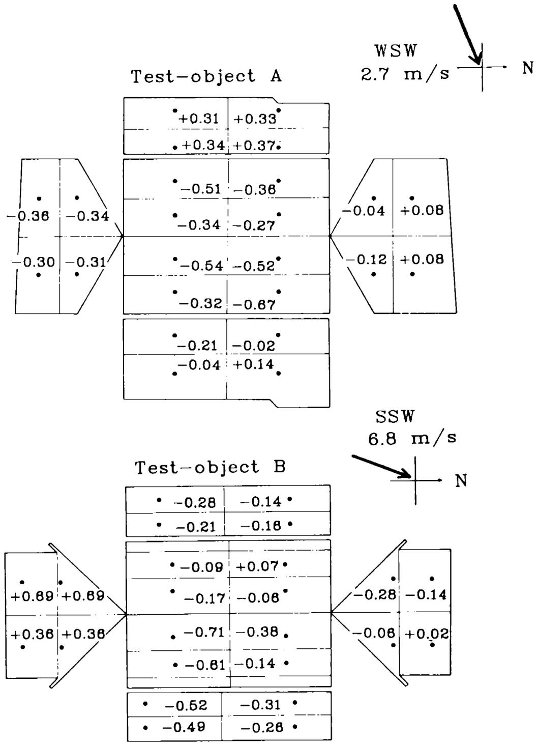
Figure 3 Pressure coefficients, measured values, [1]
