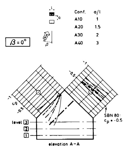
Fig. 5. Mean-pressure distributions over the test house.
