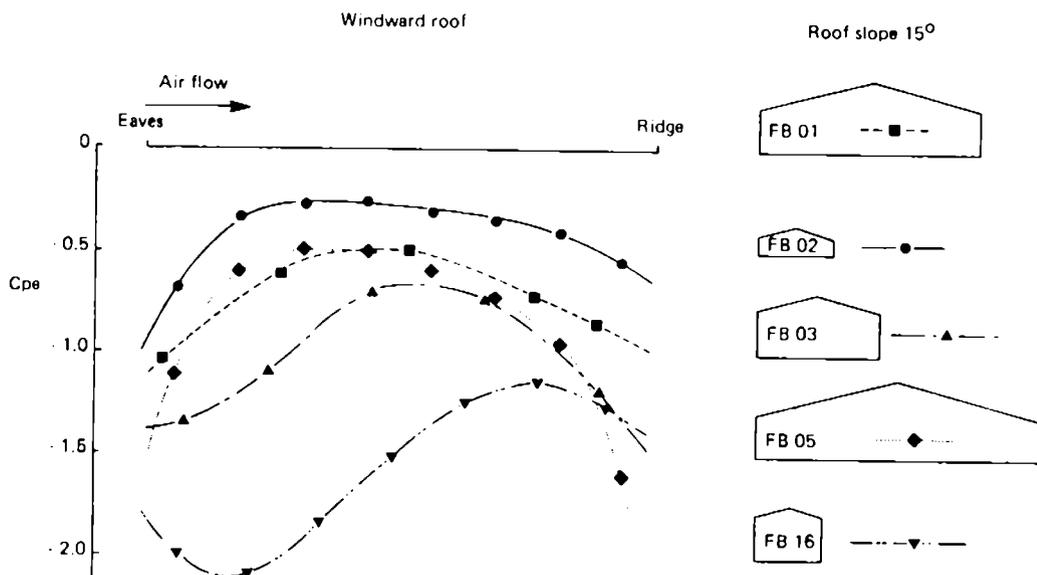
Fig. 1. Pressure distribution on the windward roof for a selection of buildings with a 15° roof slope
