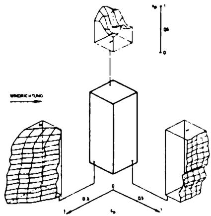
Fig.4 Isolated tall buildings - wind incident to corner
