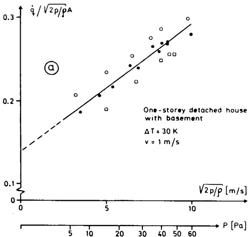
Fig. 2. Results from pressurization measurements,
