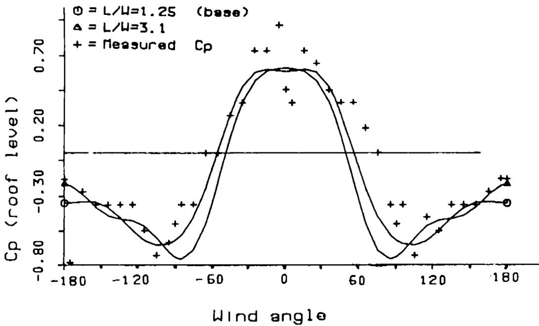
Fig. 8b Measured and calculated pressure coefficients plotted against wind angle for position 18 (end wall).
