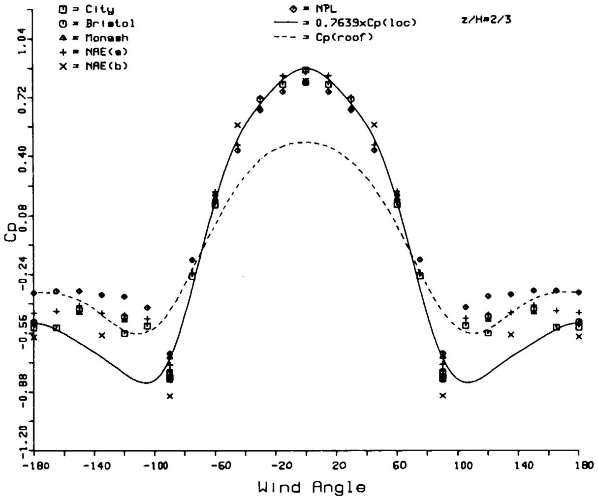
Fig. 13 Measured and calculated pressure coefficients plotted against wind angle for the CAARC Standard Tall Building Model.
