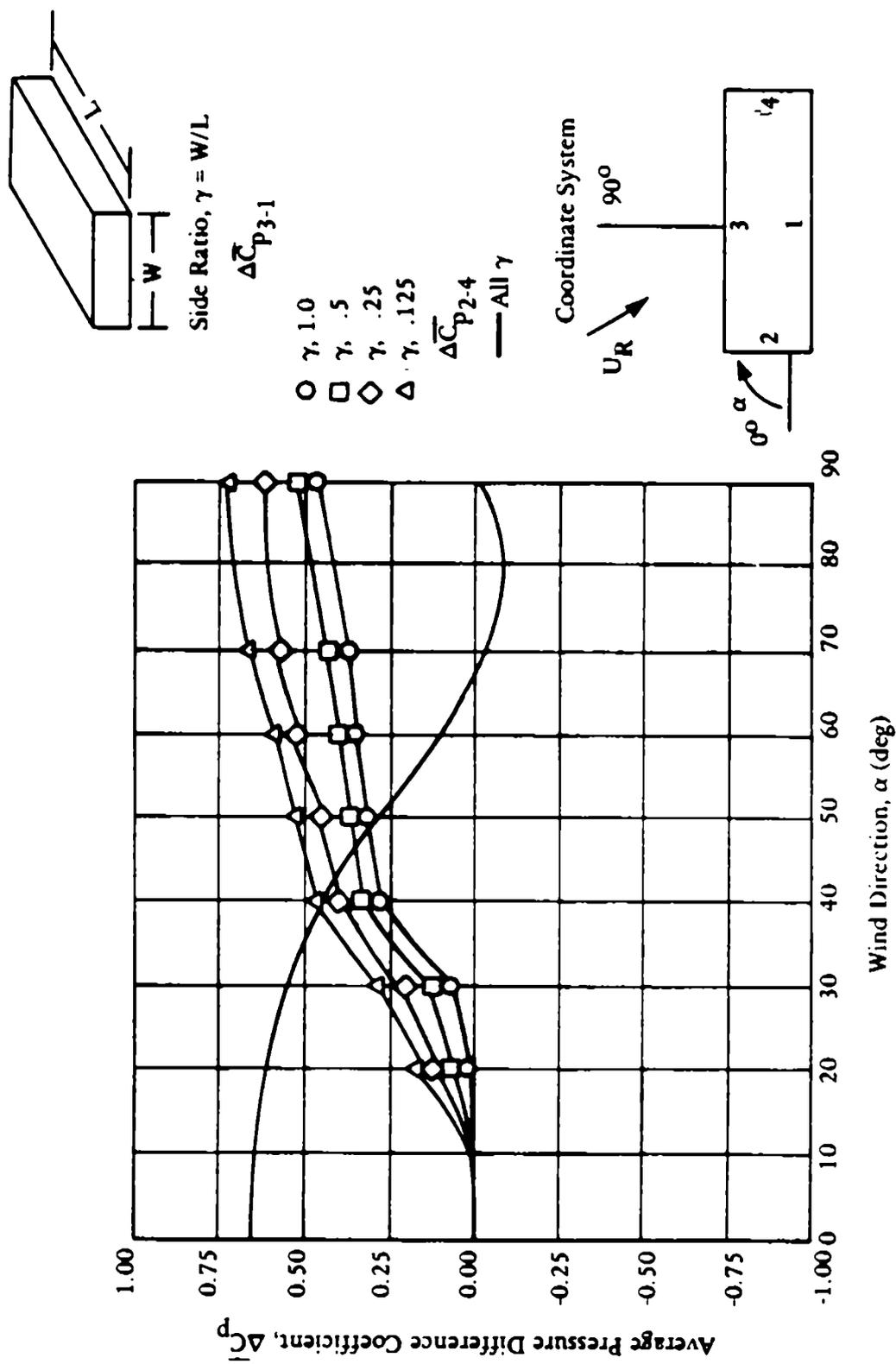
Figure 1(2) Average pressure difference coefficient for a single-story, on-grade, flat-roof rectangular building.  $\Delta \bar{C}_{P2-1}$  and  $\Delta \bar{C}_{P2-4}$  is the pressure difference coefficient between long and short walls of the building.
