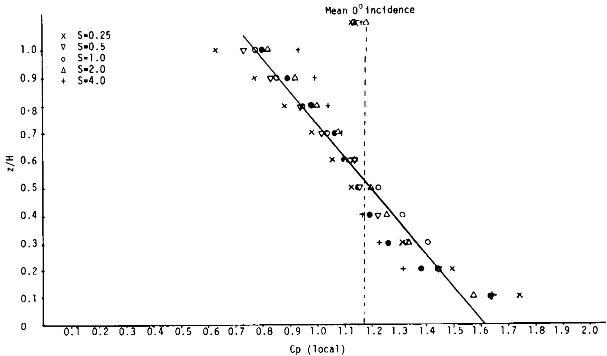
Fig. 10 Local pressure coefficients for zero wind angle and various S plotted against z/H.
