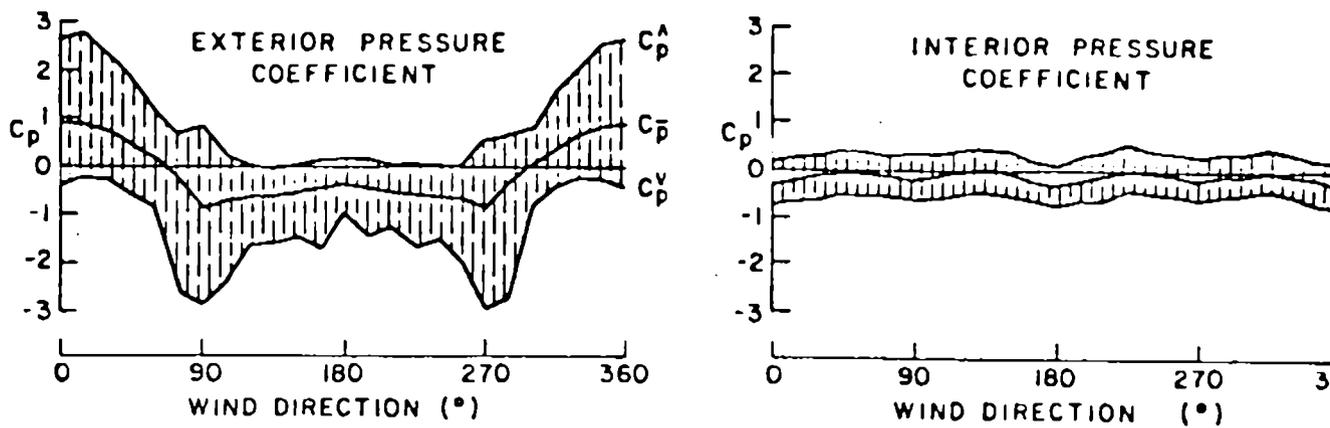
**FIG. 4** COMPARISON OF INTERNAL AND EXTERNAL PRESSURE COEFFICIENTS
