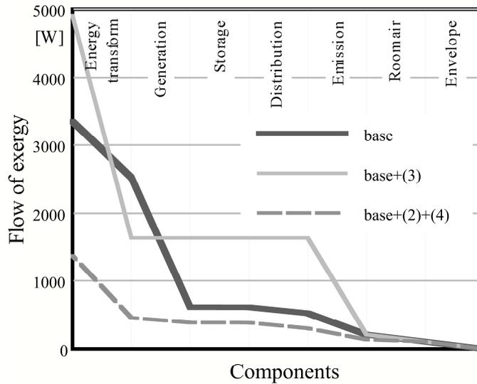
**Figure 2.** Comparison of exergy consumption for different system configurations with regard to overall system design flexibility (Schmidt & Shukuya 2003).
