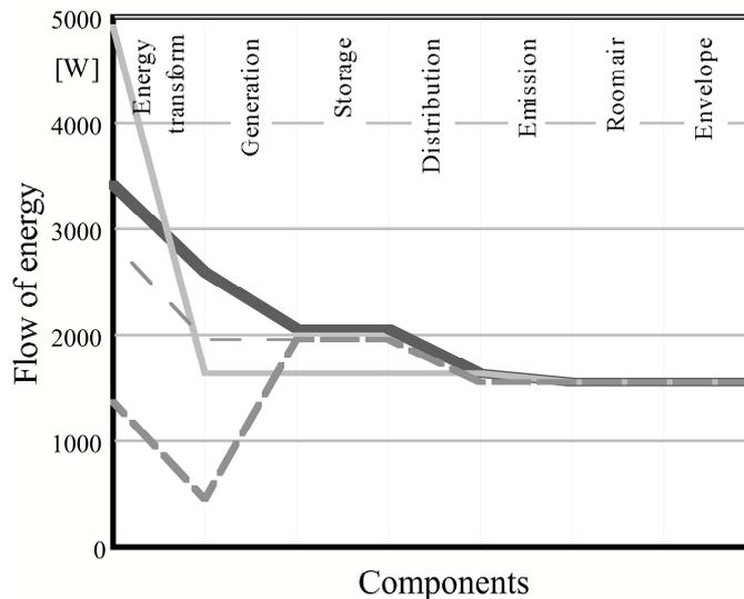
**Figure 3.** Comparison of energy utilization for different system configurations with regard to overall system design flexibility. Thin line indicates the energy flow including extracted heat from the surroundings (Schmidt & Shukuya 2003).
