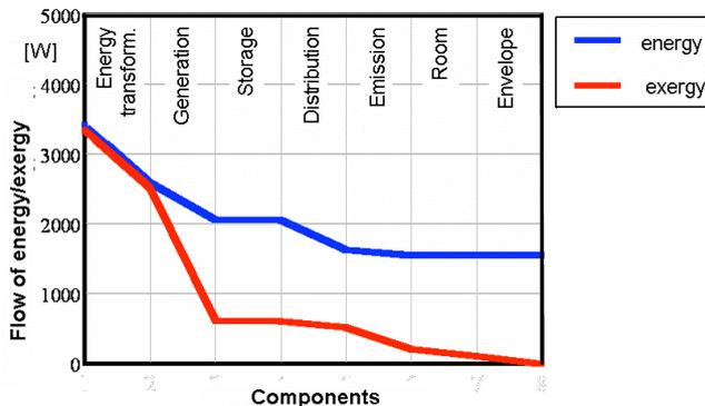
Figure 4: Results from a simplified tool for exergy analyses (Schmidt 2004)
