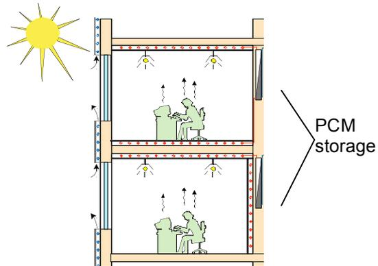
Figure 3: Active exterior façade construction for active night cooling in combination with PCM storages in the building construction
