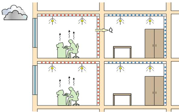
Figure 2: Displacement of heat between rooms with different thermal loads (e.g. North-South, server rooms) with capillary tube systems
