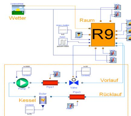
Figure 5: Detailed dynamic model for system optimisation
