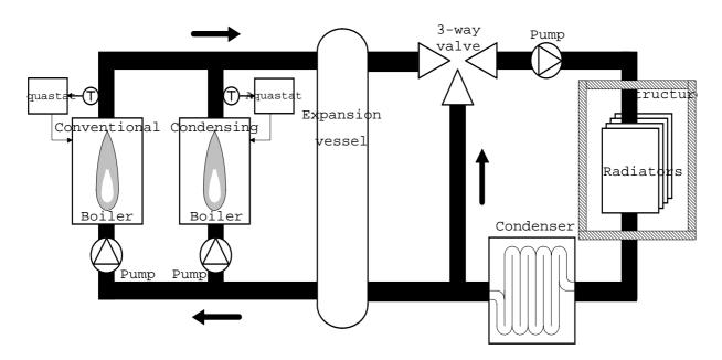
Figure 1: Diagram of the heating loop
