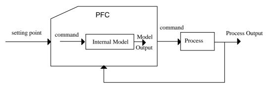
Figure 2: principle of PFC control
