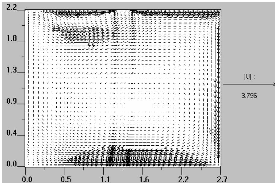
A - case #1, average and maximum velocities in the occupied zone:  $U_{avr} = 0.15$  m/s;  $U_{max} = 0.41$  m/s
