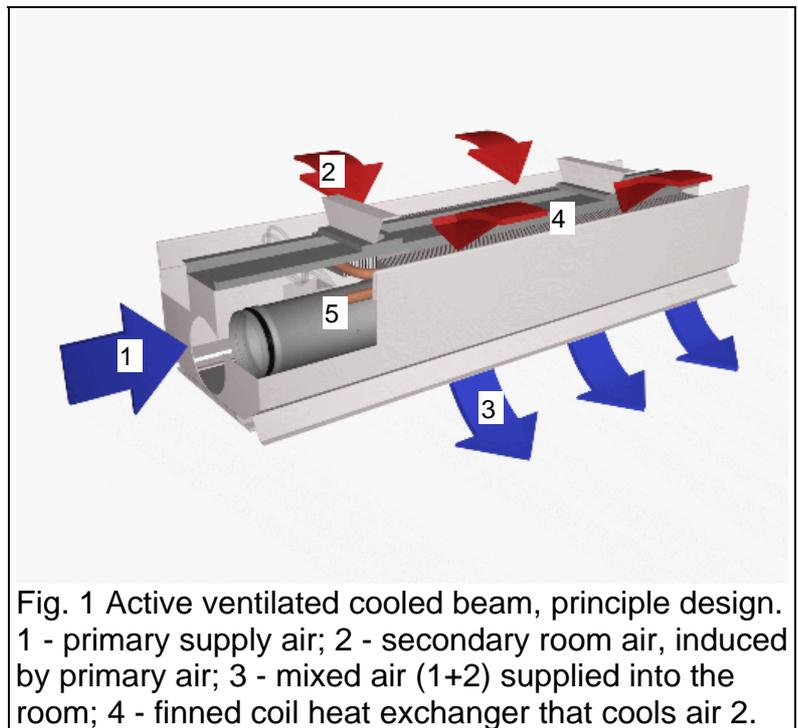
Fig. 1 Active ventilated cooled beam, principle design. 1 - primary supply air; 2 - secondary room air, induced by primary air; 3 - mixed air (1+2) supplied into the room; 4 - finned coil heat exchanger that cools air 2.
