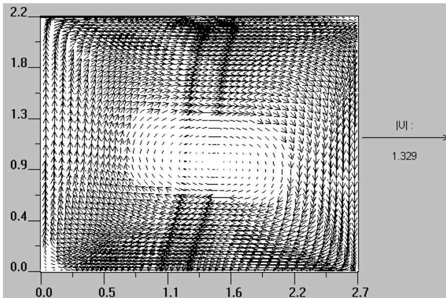
B - case #2, average and maximum velocities in the occupied zone:  $U_{avr} = 0.16$  m/s;  $U_{max} = 0.4$  m/s
