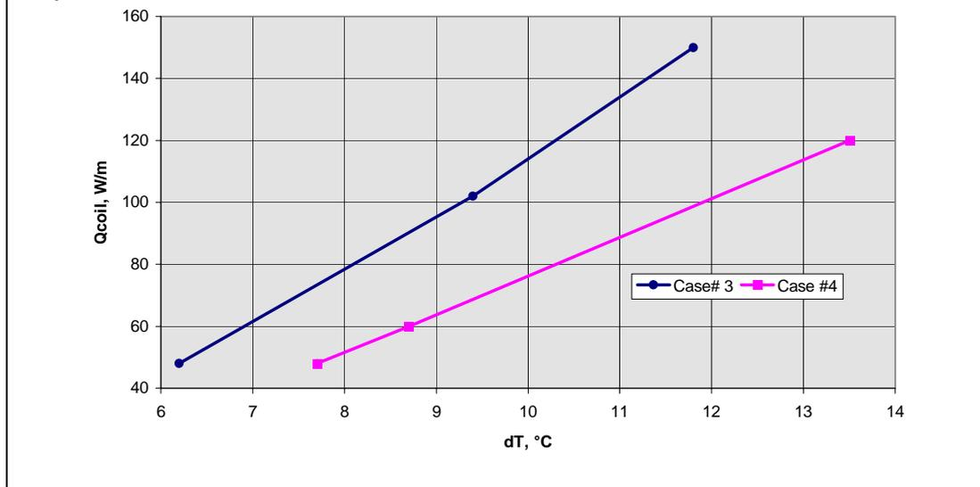
Fig. 6 Cooling capacity of the static beam  $Q_{coil}$  as function of temperature difference  $dT$
